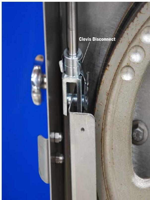
Figure 6. Quick Disconnect Clevis
