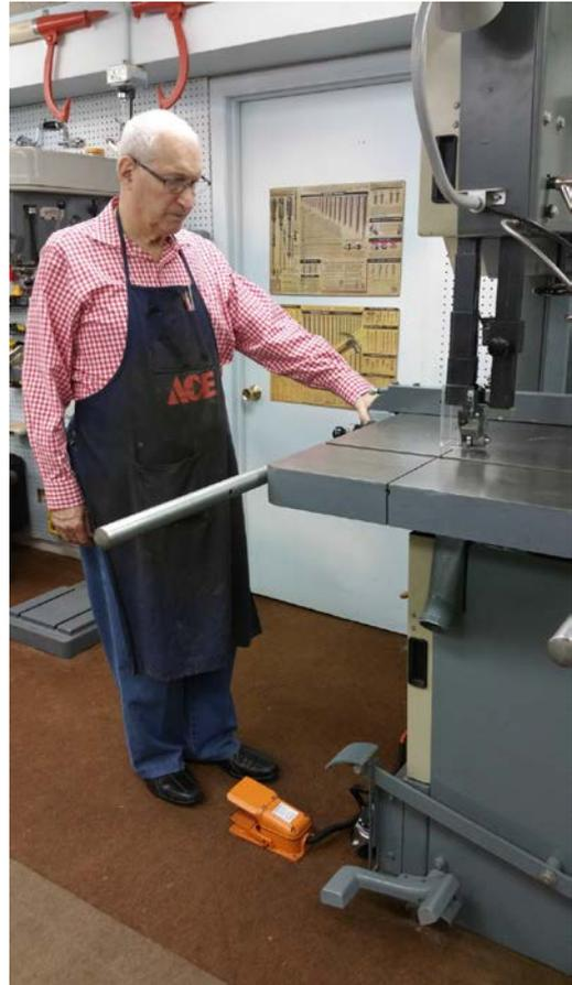
**Figure 14.** Fully Guarded Band Saw Blade, Pedal is not Depressed
