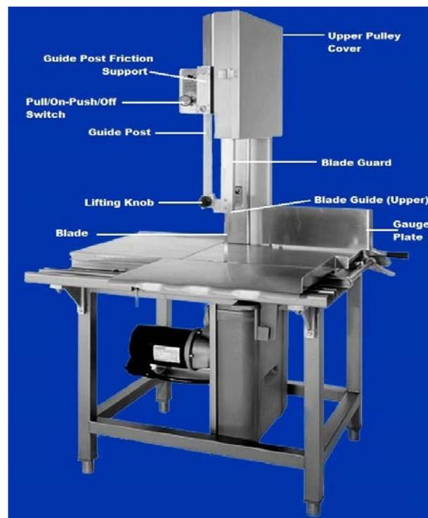
Figure 1. Typical Meat-Cutting Vertical Band Saw
