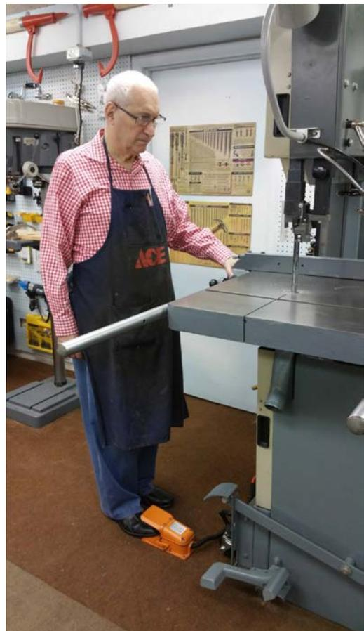
**Figure 15.** Exposed Band Saw Blade for Cutting
