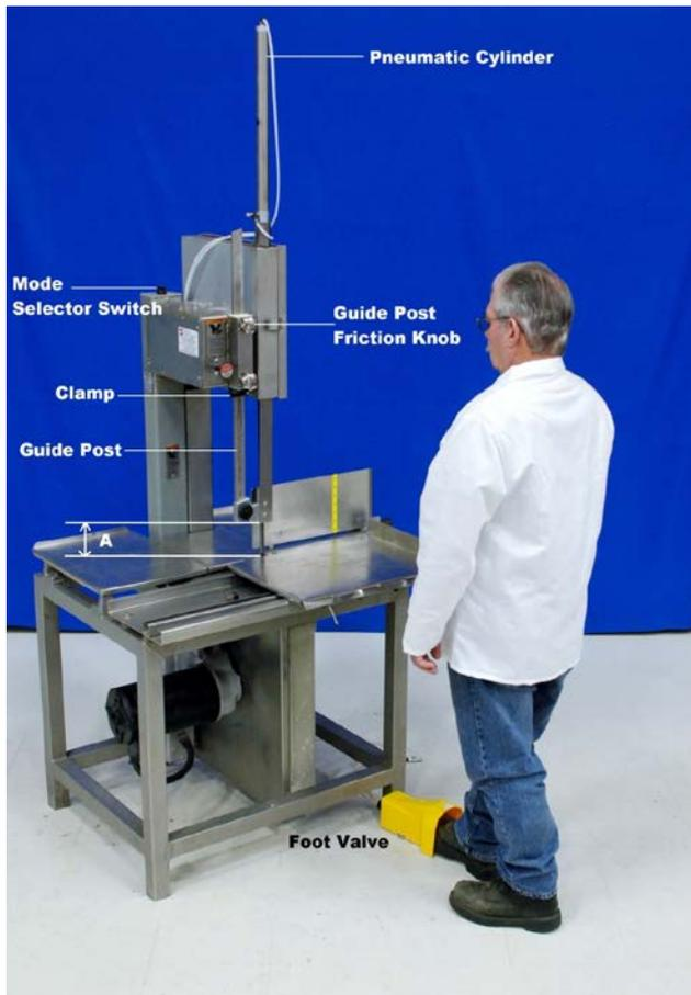
**Figure 3.** Retrofit Meat Saw with Depressed Foot Pedal— Pneumatic cylinder exposes blade height = A
