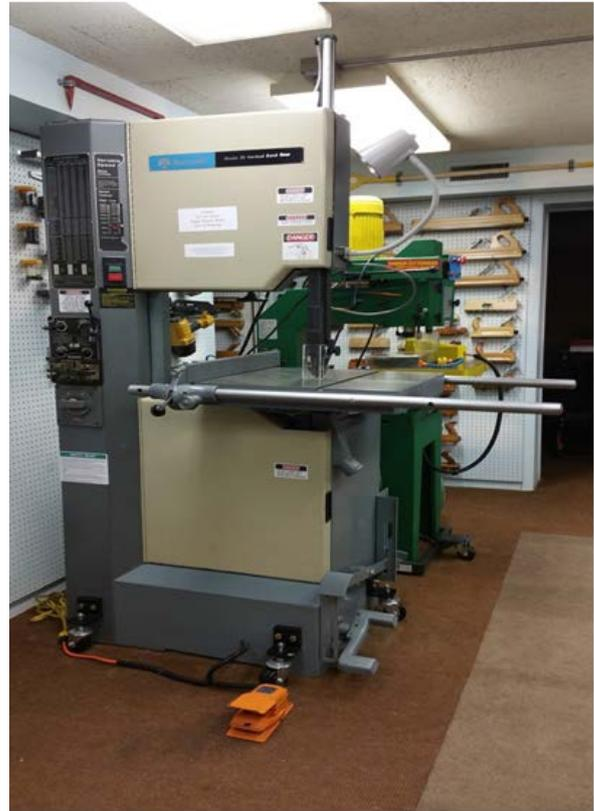
Figure 8. Rockwell 20" Metal-Wood Vertical Band Saw
