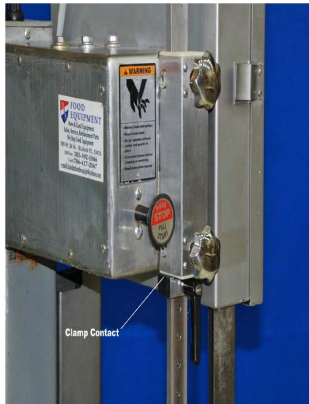
**Figure 4.** Retrofit Controls: Push Stop/Pull Start, Two Friction Knobs, Clamp
