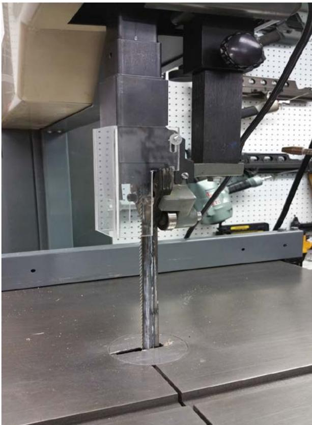
**Figure 11.** Contact Between the Clamp and the Bottom of the Guide Post Support Bracket
