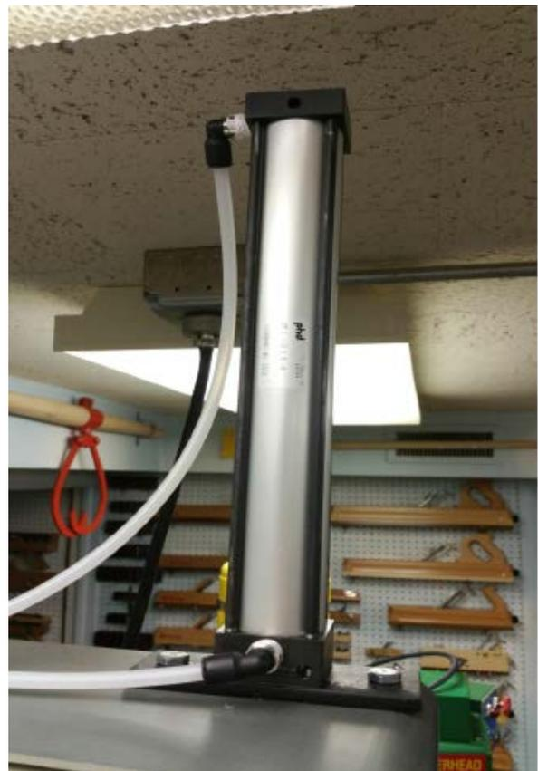
Figure 9. Two-Way Pneumatic Cylinder
