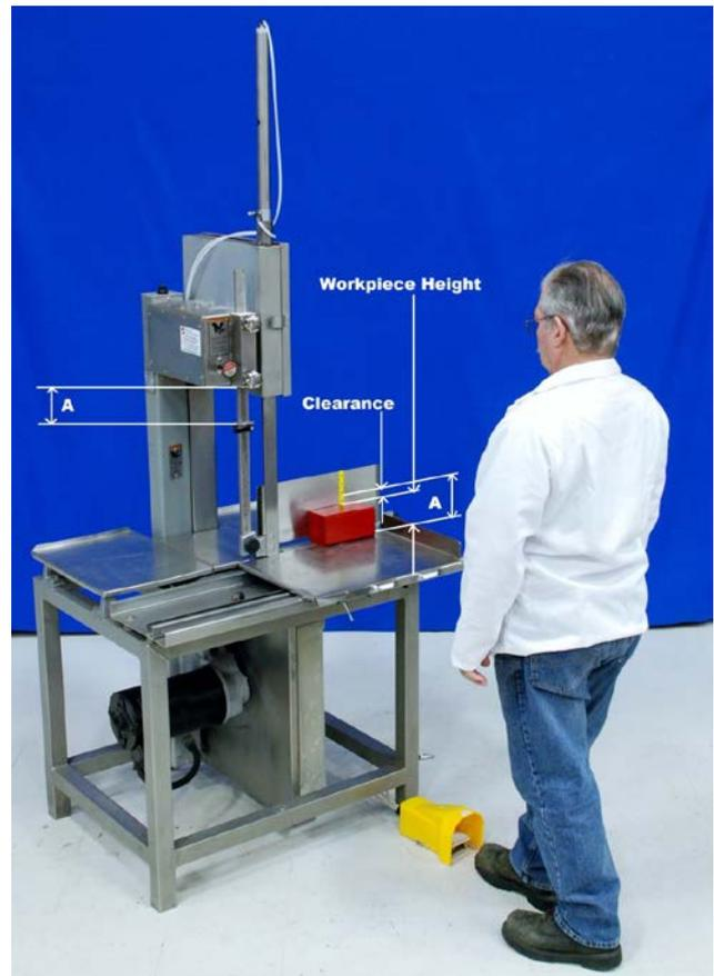
**Figure 2.** Retrofit Meat Saw With Foot Pedal Released— Workpiece height plus clearance = A; Clamp setting = A; Guard touches table top
