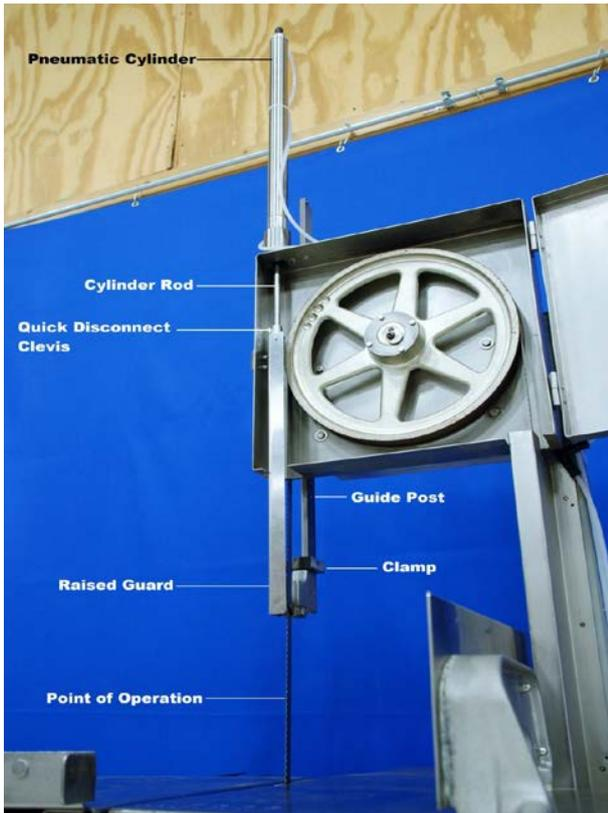
Figure 5. The Linkage: Cylinder, Cylinder Rod, Quick Disconnect Clevis, L-Shaped Guard, Guide Post, Clamp, Blade
