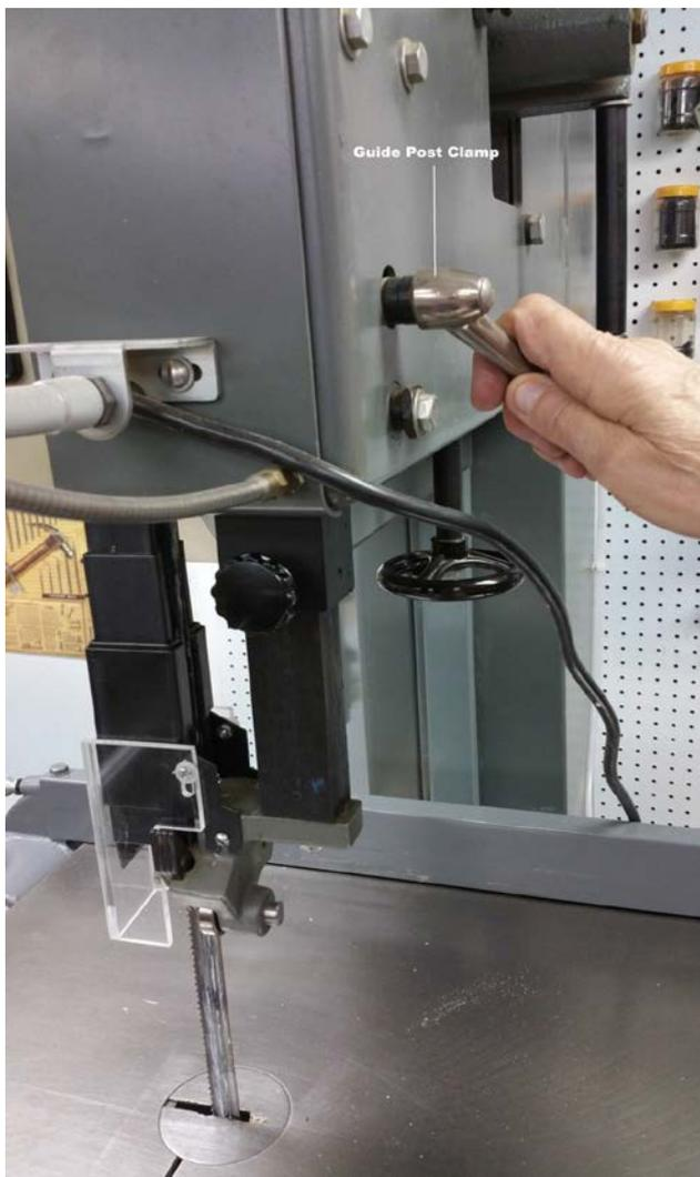
Figure 16. Original Guide Post Clamp
