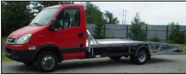
**Figure 5.** Real breakdown truck body construction fixed on required vehicle for this particular case
