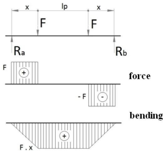
Figure 4. Graphical interpretation of the loaded beam
