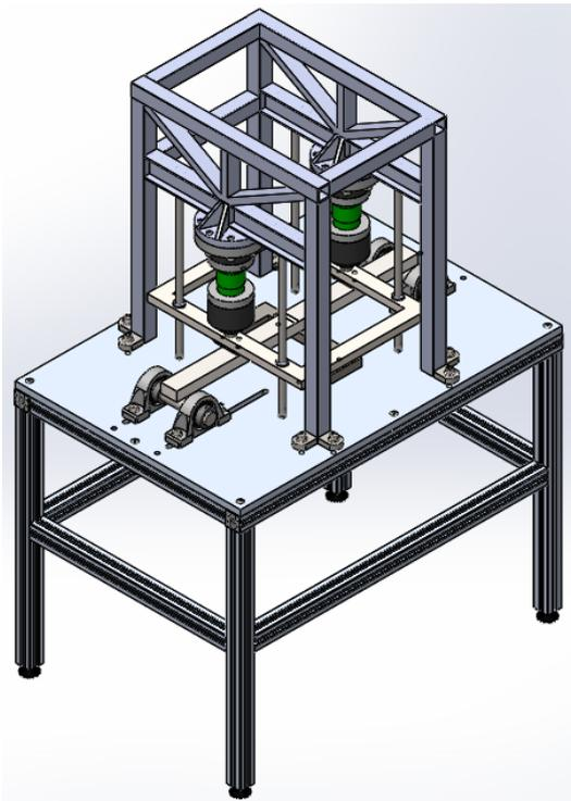
Figure 11. Final design of the bend testing machine
