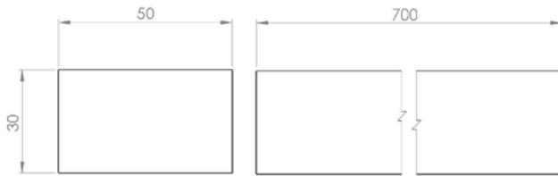
Figure 2. Specimen: front view, side view
