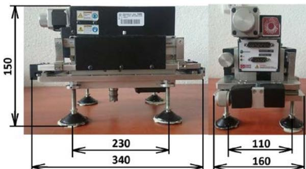
Figure 1. MTS - 3000 Ring-Core system
