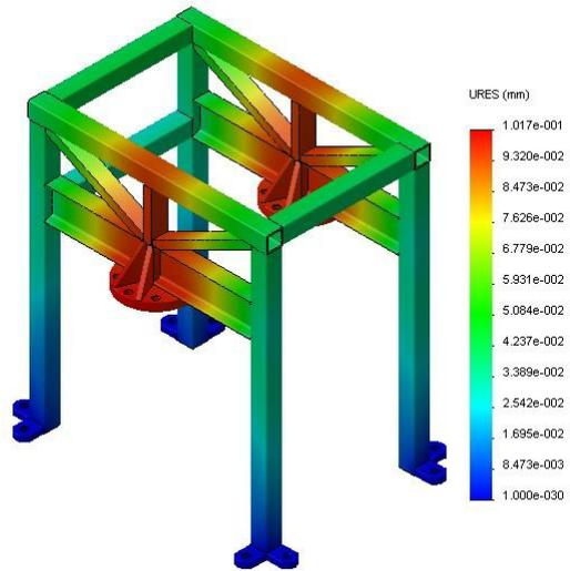
Figure 7. Simulation of the displacement on the frame
