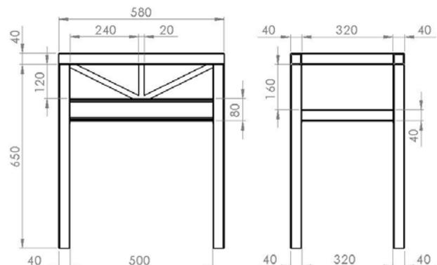
Figure 5. Frame dimensions of the bending device
