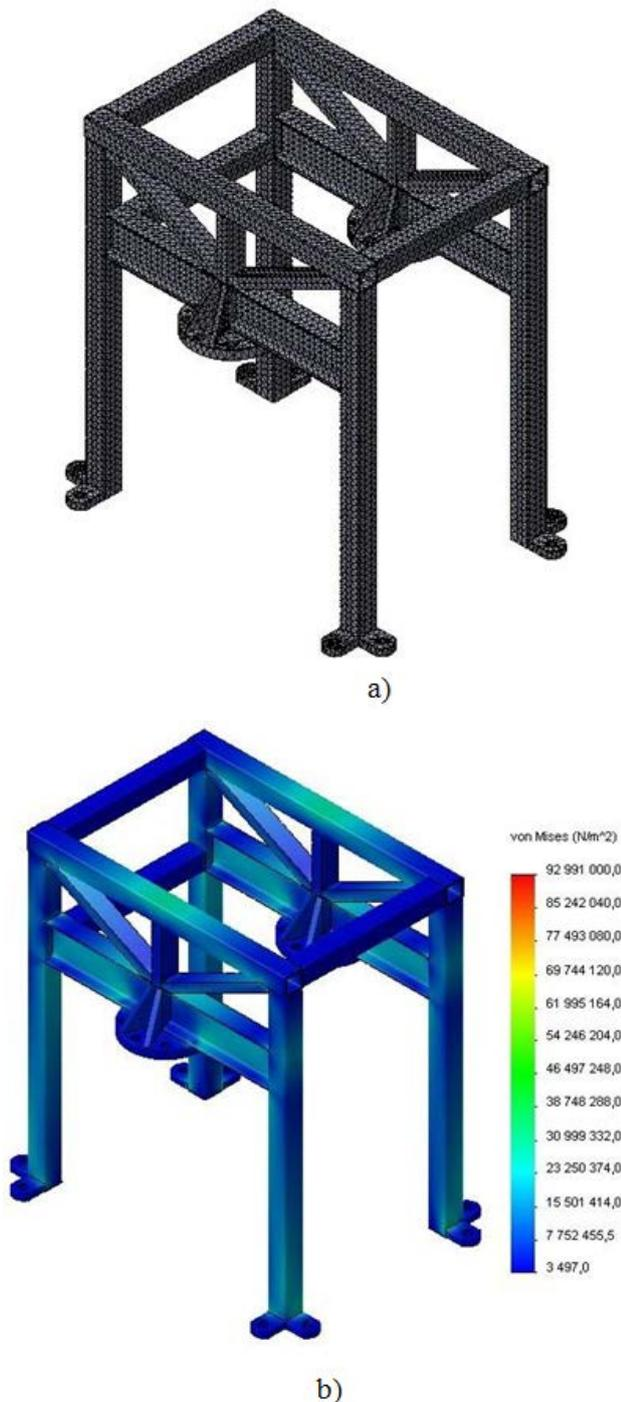
Figure 6. a) Mesh model of the frame b) Simulation of the stresses of the frame
