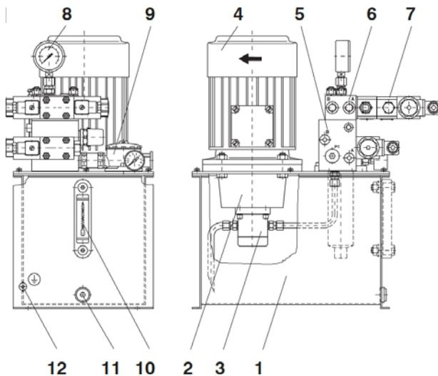
1 – tank, 2 – drive/bell housing, 3 – pump, 4 – electric motor, 5 – base block (safety block of the accumulator), 6 – horizontal stacking assembly, 7 – vertical stacking assembly, 8 – pressure gauge, 9 – return filter with by-pass, integrated air breather/filler and clogging indicator, 10 – continuous level gauge, 11 – magnetic drain plug, 12 – grounding point
