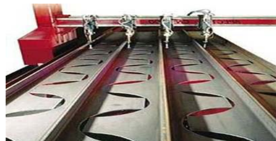
Figure 2. Flame cutting of rolled sections for circular holes
