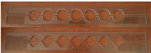
Figure 4. Beam models made from photosensitive material PSM-1
