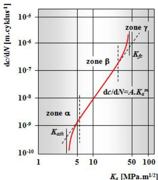
Figure 4. The kinetic diagram of fatigue damage
