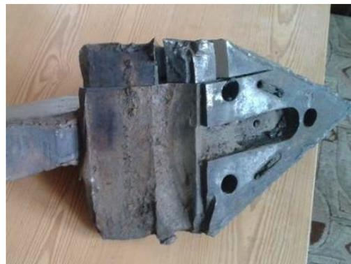
Figure 5. The overview of the failures part of the holder of knife
