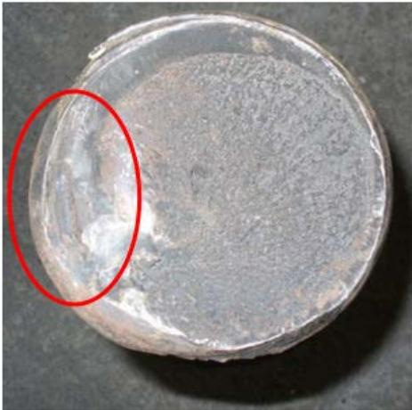
Figure 7. The fracture area of the broken part of the turbine shaft
