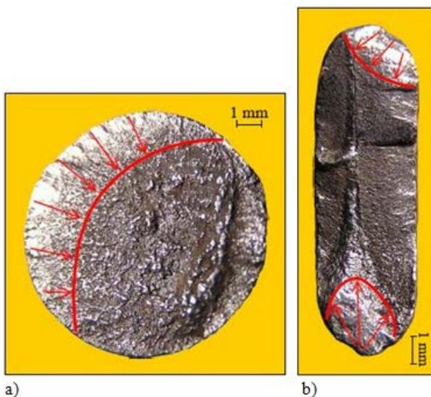
**Figure 2.** Typical surfaces of fatigue fractures caused by the real load
