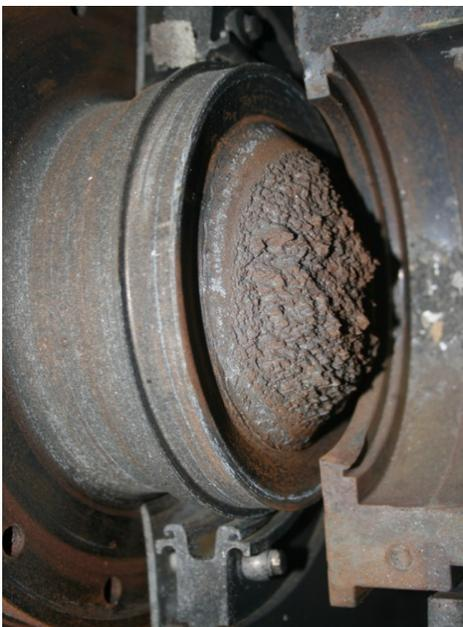
Figure 8. The fracture area of the opposite broken part of the turbine shaft
