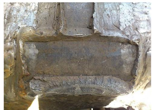
Figure 6. The shaft after the failure of the holder of a crusher moving knife
