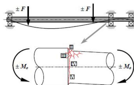
**Figure 3.** The phases of the fatigue process
