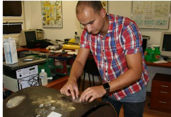
Figure 6. Application of two-component adhesive and photoelastic material on a pipeline
