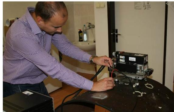
Figure 7. Drilling with SINT-MTS 3000 Ring-Core
