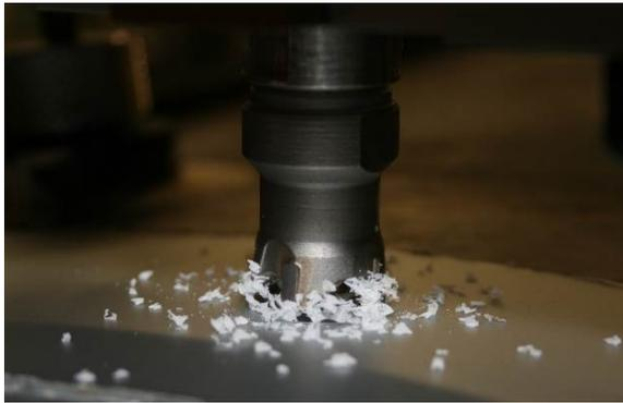
**Figure 9.** Milling into photoelastic material PS-1D
