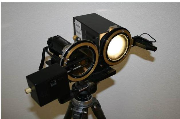
Figure 5. Reflection Polariscopes LF/Z-2
