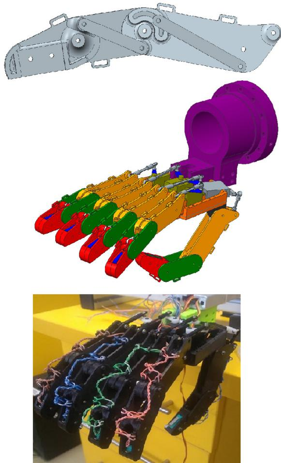
**Figure 7.** 3D model of finger and robotic hand
