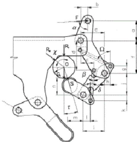
Figure 5. Forces for gripping
