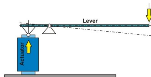
Figure 1. Lever displacement amplifier
