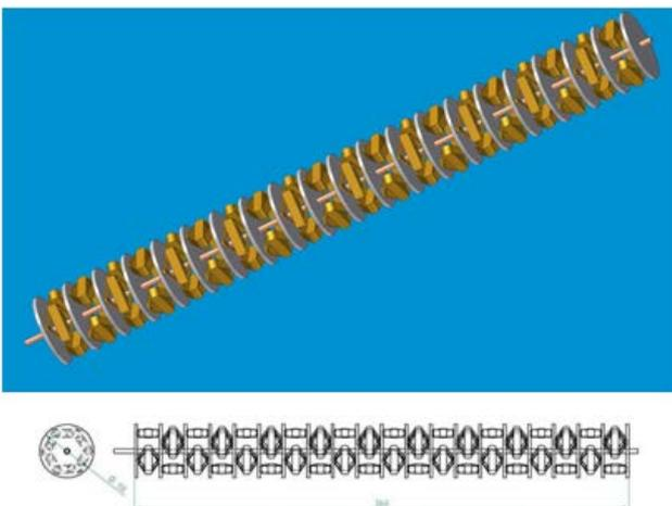
Figure 11. Composition of serial-parallel arrangement of 60 pieces of amplified piezoactuator
