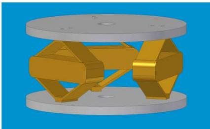
Figure 10. Block of parallel arrangement of 3 pieces of amplified piezoactuator
