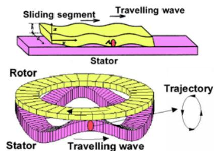
Figure 7. Principle of the planar and rotary ultrasonic motor [5]
