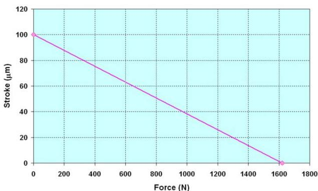
Figure 9. Characteristic of selected amplified piezoactuator
