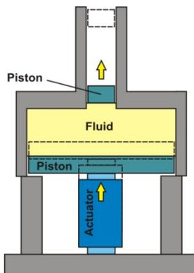
Figure 5. Hydraulic displacement amplifier
