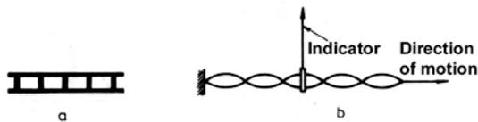
Figure 3. Displacement amplifier with deformation part
