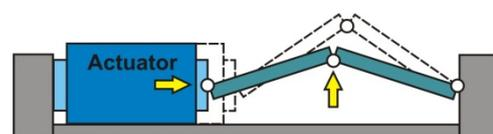
Figure 2. Flexure bridges displacement amplifier
