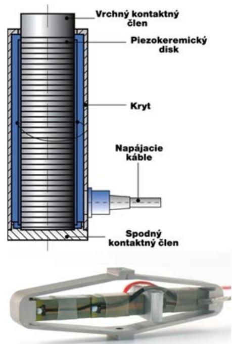
Figure 8. Piezostack and amplified piezoactuator [5]
