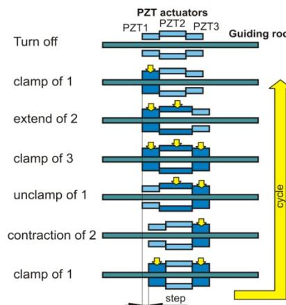
Figure 6. Inchworm motor
