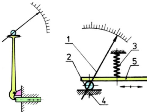
Figure 4. Gearing and friction gearing for displacement amplifying
