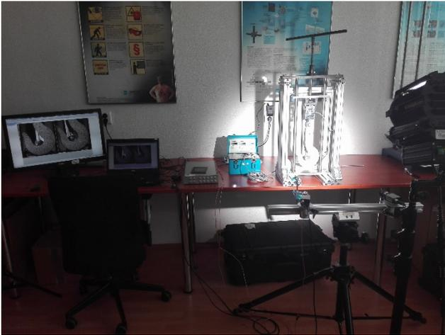
Figure 8. Measuring chain used for the realization of the experimental stress analysis via digital image correlation
