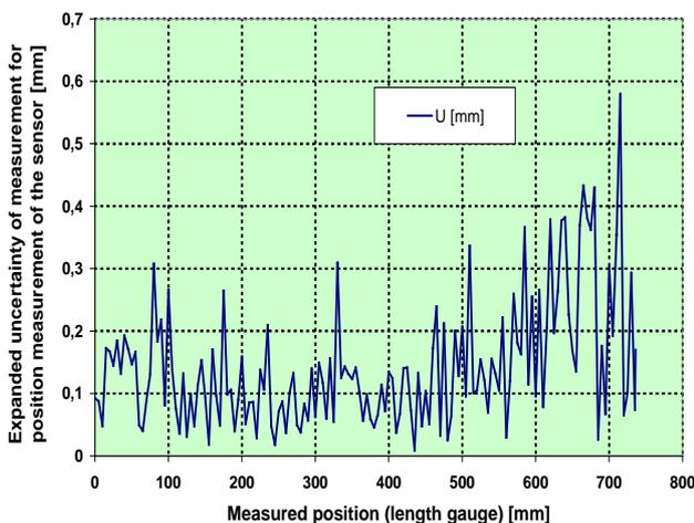
Figure 7. The expanded uncertainty of position measurement
