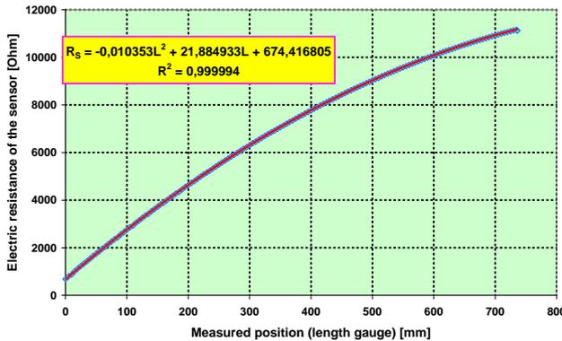
Figure 3. Position sensor static characteristic
