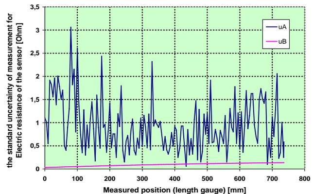
Figure 4. The standard uncertainty of measurement for electric resistance of the sensor measured in calibration process
