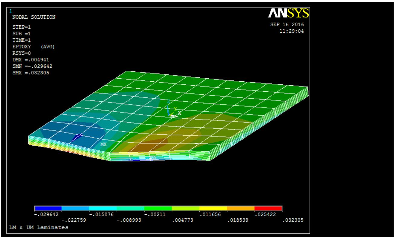
Figure 19. XY Shear Total Mechanical Strain of LM & UM [(+/-45)<sub>s</sub>]<sub>n</sub> Laminate Design
