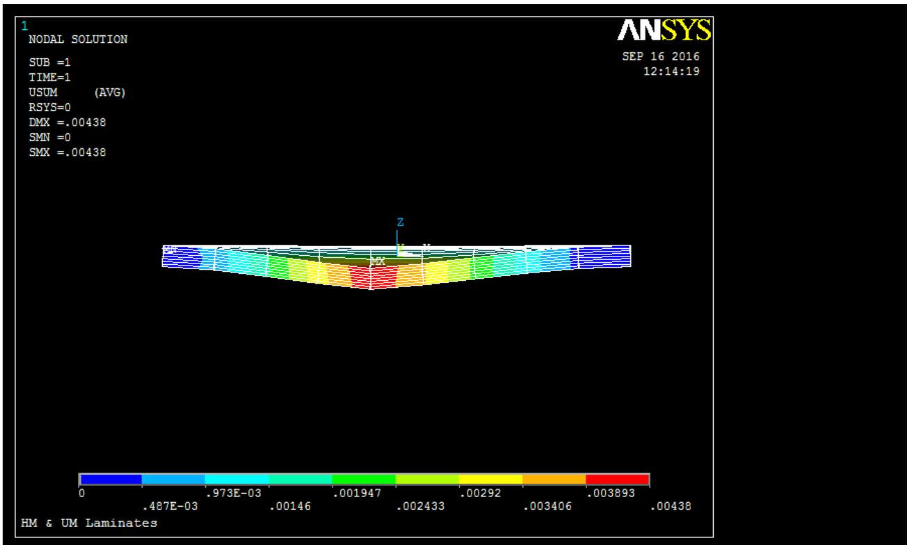
Figure 27. Deflection of HM & UM [(+/-45)s]<sub>n</sub> Laminate Design.
