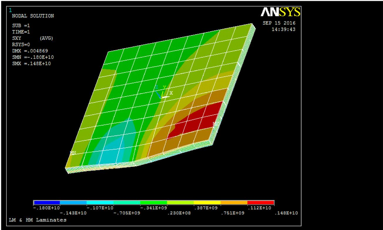
Figure 10. XY Shear Stress of [(+/-45/0/90)<sub>s</sub>]<sub>n</sub> Laminate Design.
