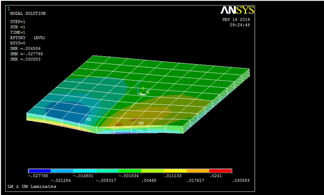
Figure 18. XY Shear Total Mechanical Strain of LM & UM [(+/-45/0/90)<sub>s</sub>]<sub>n</sub> Laminate Design.
