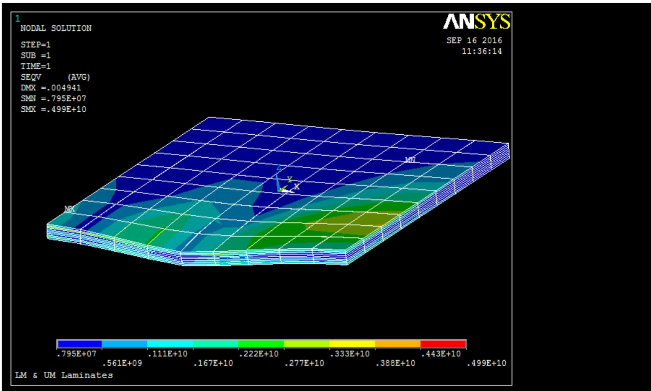
Figure 23. Von Mises Stress of LM & UM [(+/-45)s]<sub>n</sub> Laminate Design.
