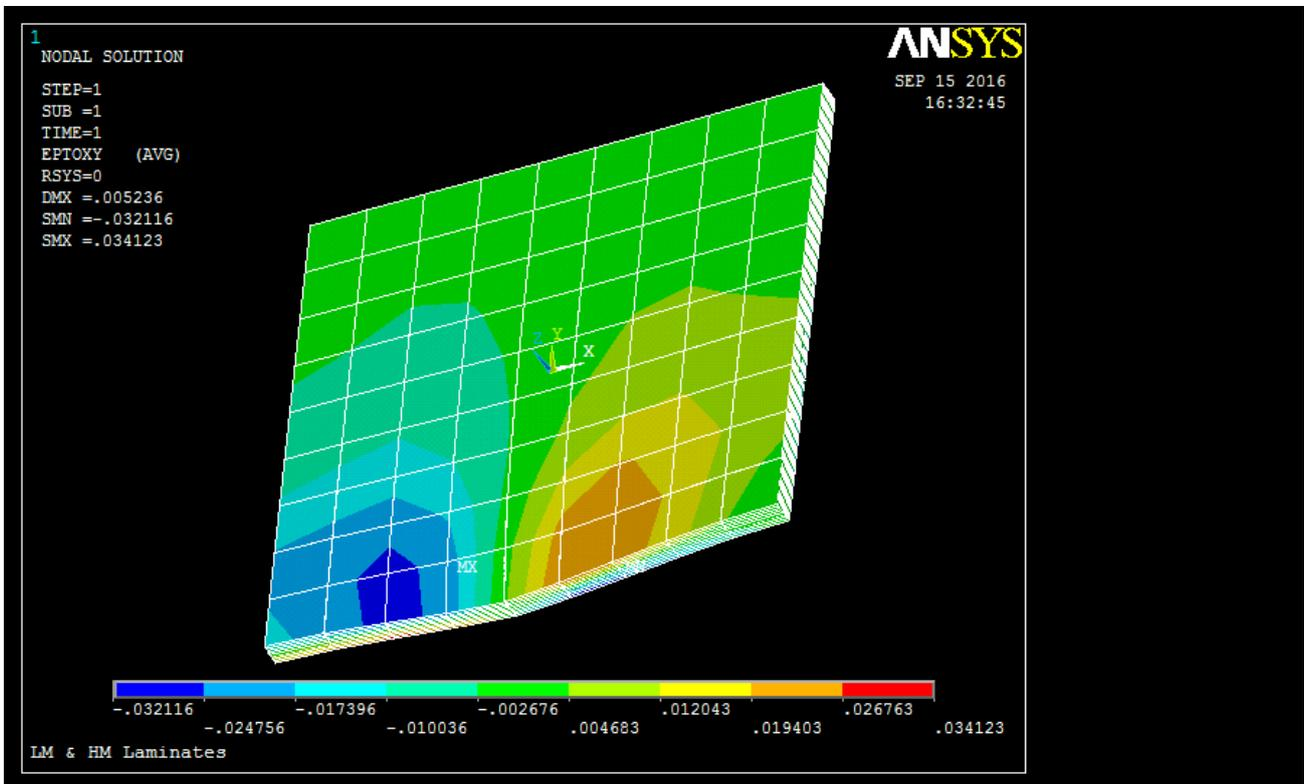
Figure 9. XY Shear Total Mechanical Strain of [(+/-45)s]n Laminate Design.
