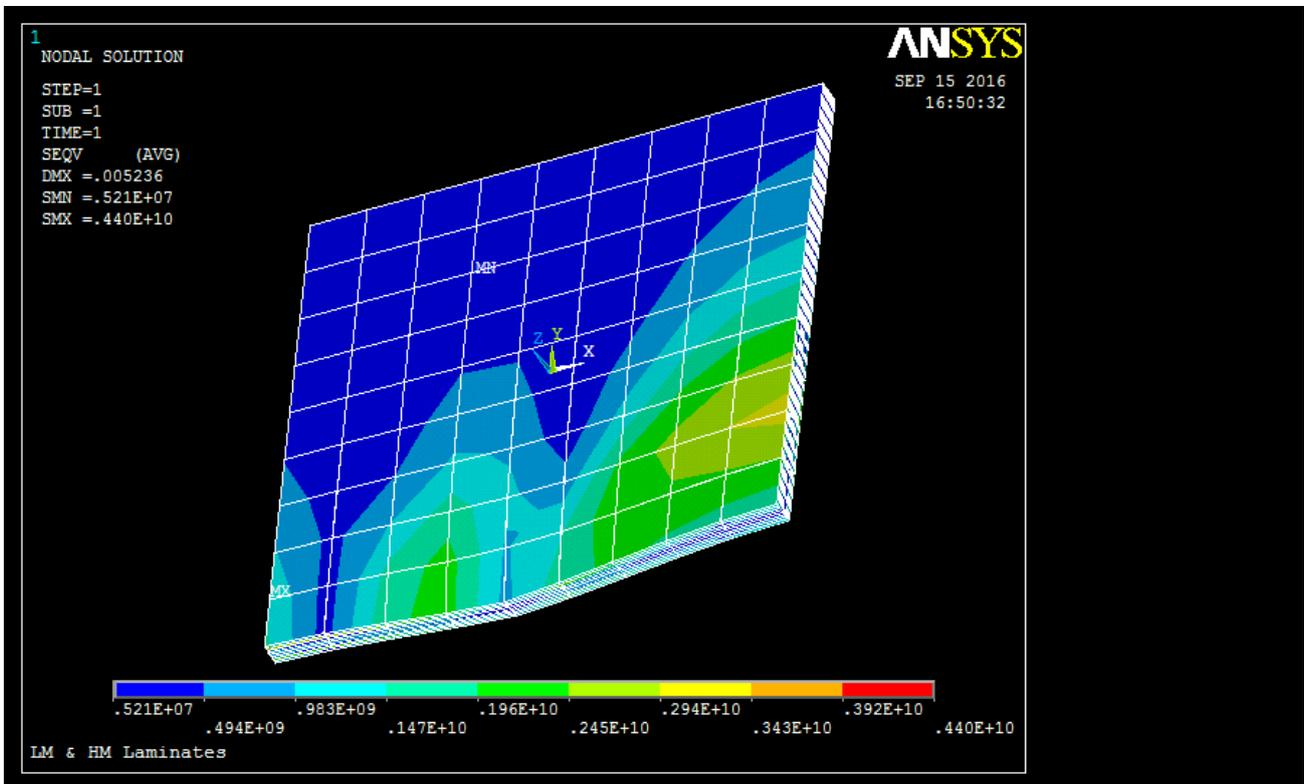
Figure 13. Von Mises Stress of  $[(+/-45)_s]_n$  Laminate Design.
