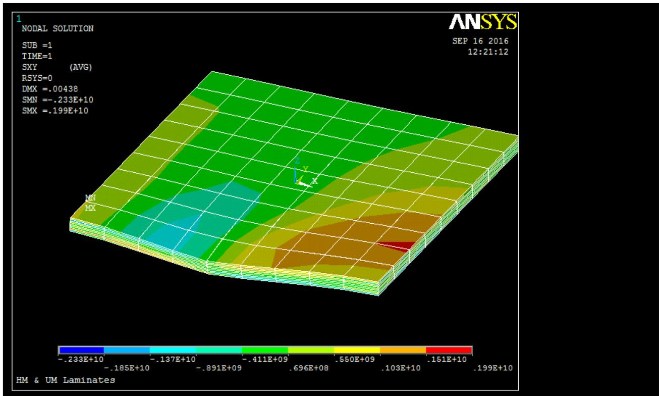
Figure 31. XY Shear Stress of HM & UM [(+/-45)s]n Laminate Design.
