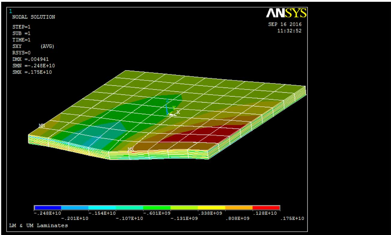
Figure 21. XY Shear Stress of LM & UM [+/-45]s<sub>n</sub> Laminate Design.
