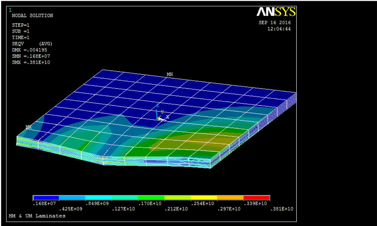
Figure 32. Von Mises Stress of HM & UM [(+/-45/0/90)s]<sub>n</sub> Laminate Design.
