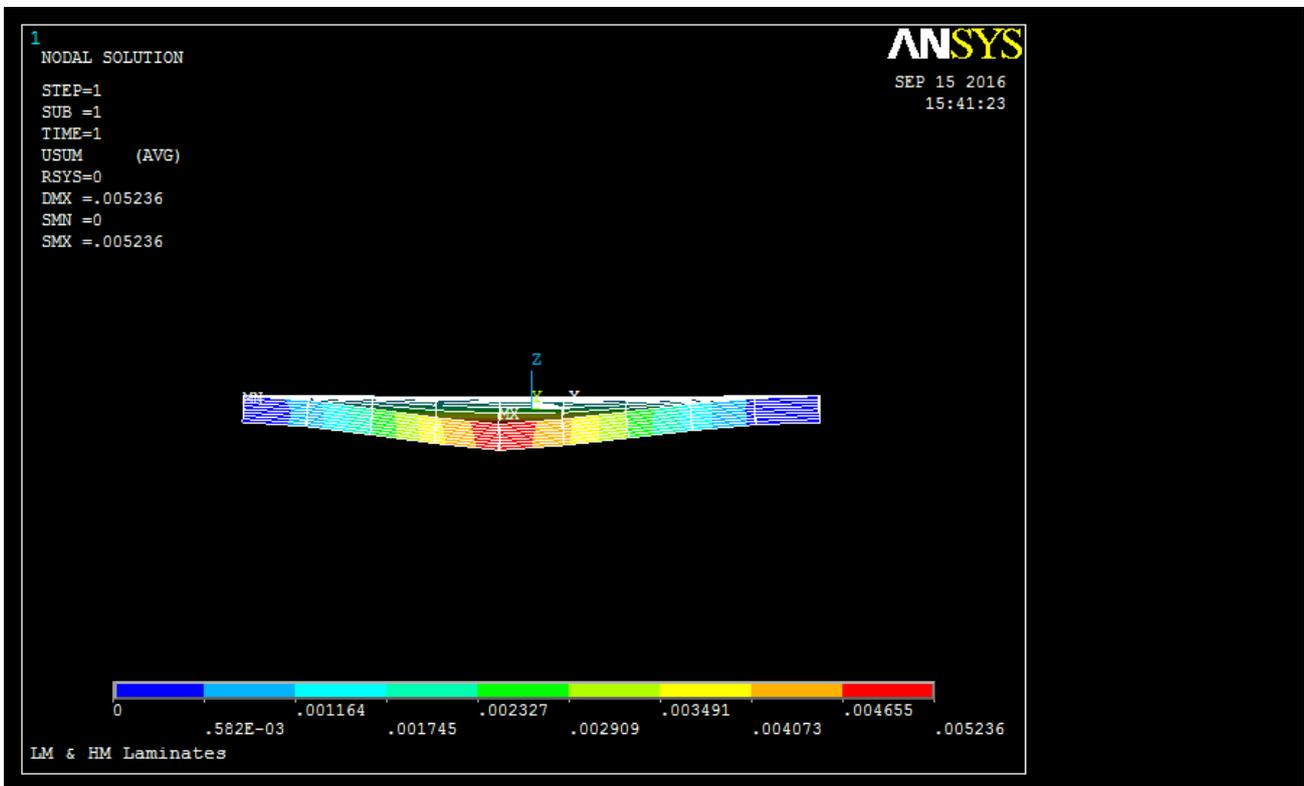
Figure 7. Deflection of [(+/-45)s]n Laminate Design.
