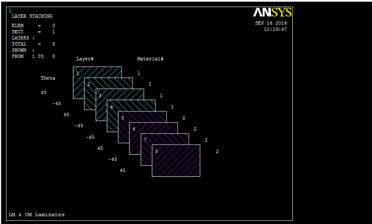
Figure 15. [(+/-45)<sub>s</sub>]<sub>n</sub> LM & UM Laminate Design Stacking Sequence.
