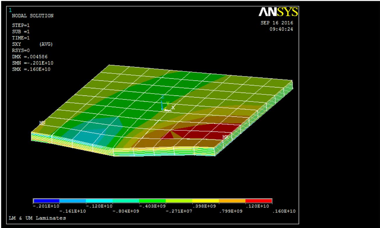
Figure 20. XY Shear Stress of LM & UM [+/-45/0/90]s<sub>n</sub> Laminate Design.
