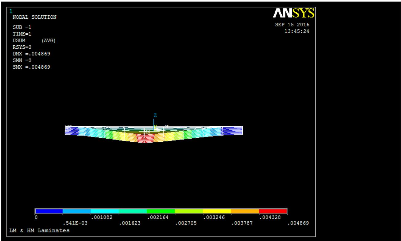
Figure 6. Deflection of [(+/-45/0/90)s]n Laminate Design.
