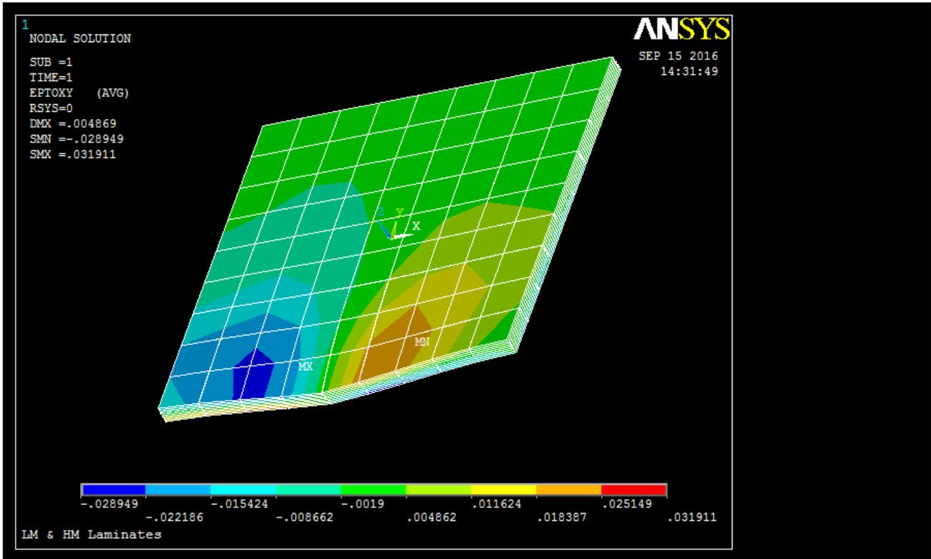
Figure 8. XY Shear Total Mechanical Strain of [(+/-45/0/90)s]n Laminate Design.
