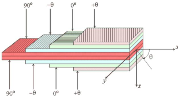
Figure 1. Laminate with stacking sequence  $[\theta, 0, -\theta, 90]_s$
