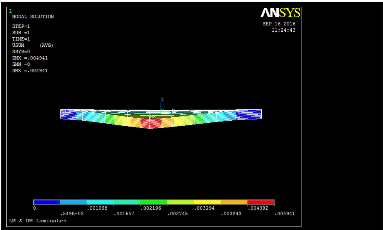
Figure 17. Deflection of LM & UM [(+/-45)s]<sub>n</sub> Laminate Design.
