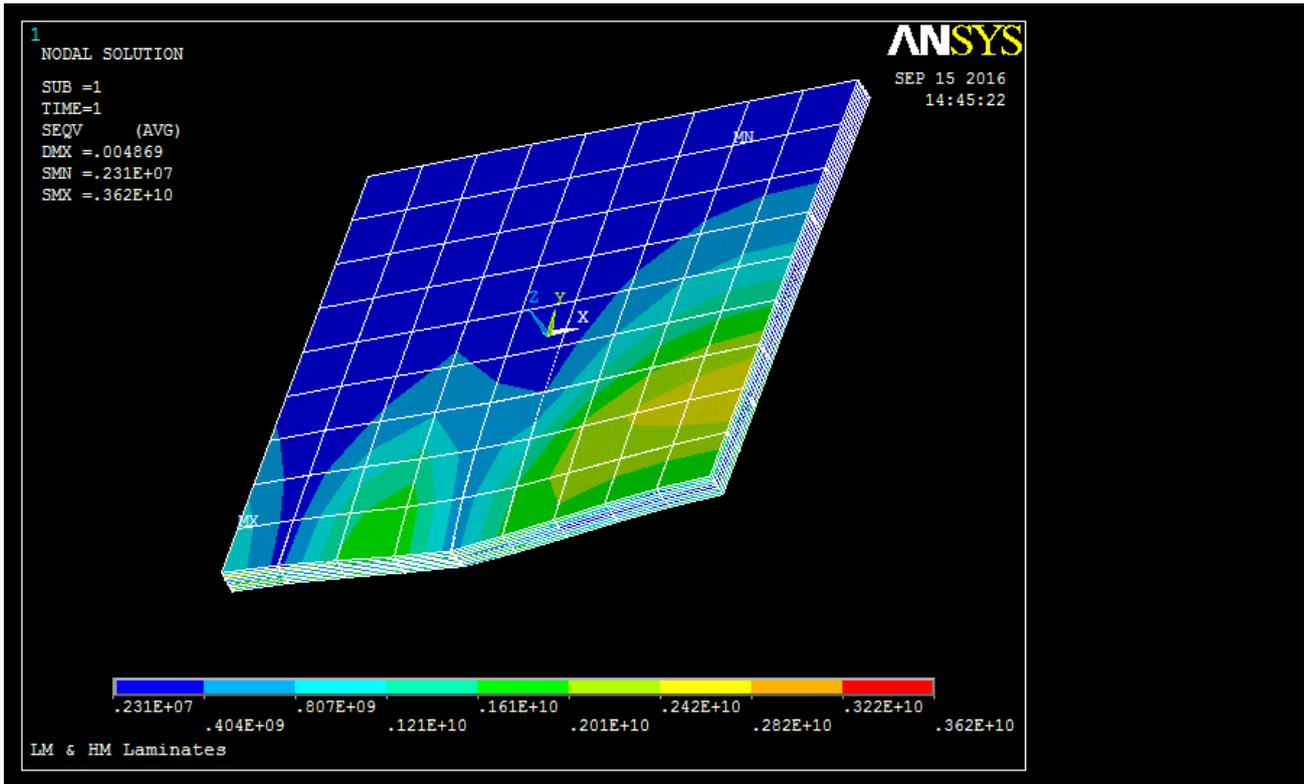
Figure 12. Von Mises Stress of  $[(+/-45/0/90)_s]_n$  Laminate Design.
