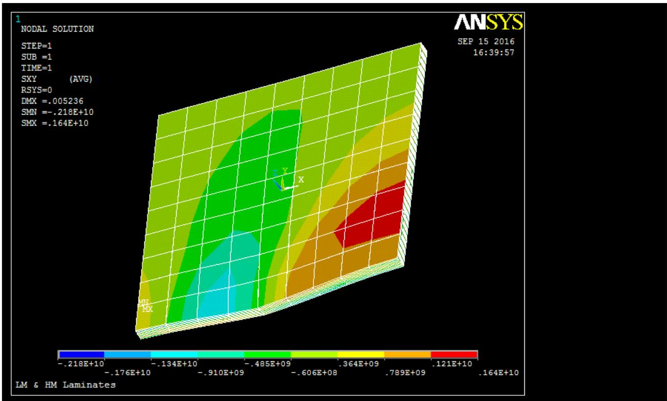
Figure 11. XY Shear Stress of [(+/-45)<sub>s</sub>]<sub>n</sub> Laminate Design.
