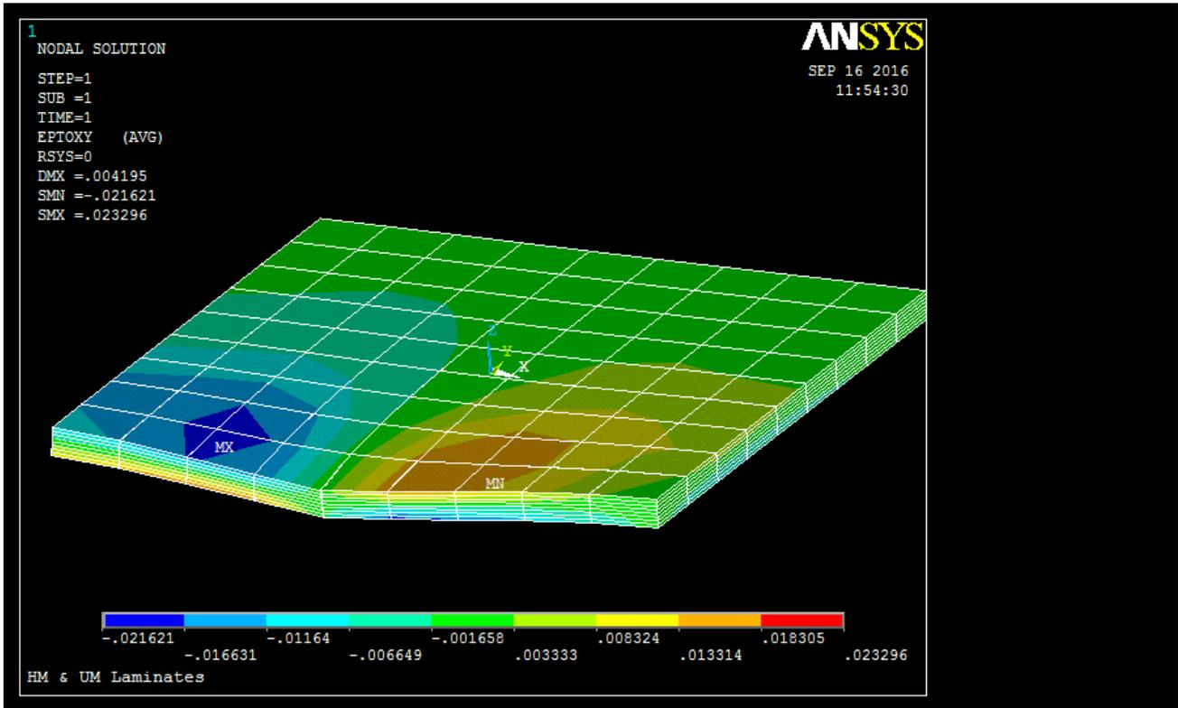
Figure 28. XY Shear Total Mechanical Strain of HM & UM [(+/-45/0/90)s]<sub>n</sub> Laminate Design.
