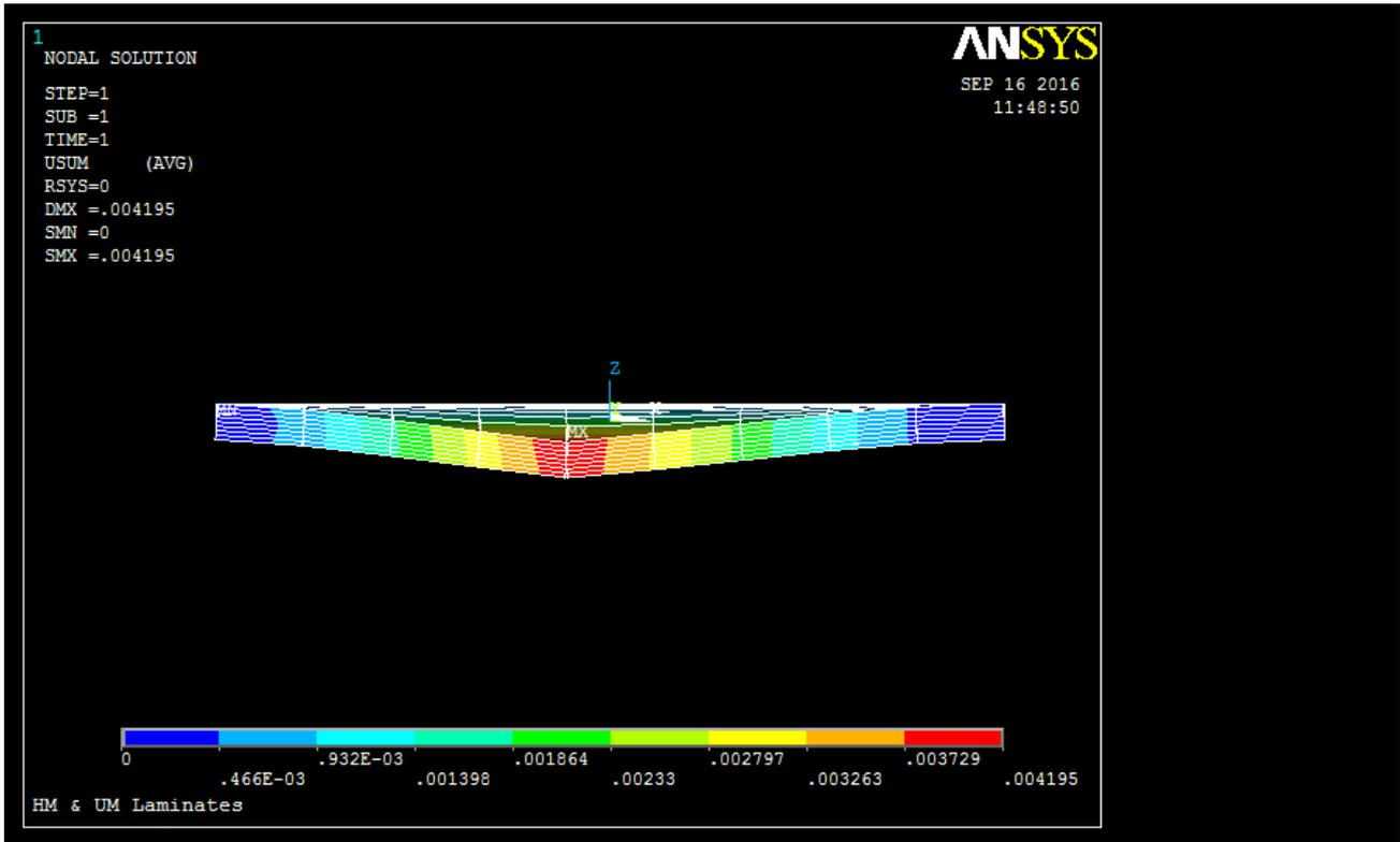
Figure 26. Deflection of HM & UM [(+/-45/0/90)s]<sub>n</sub> Laminate Design.
