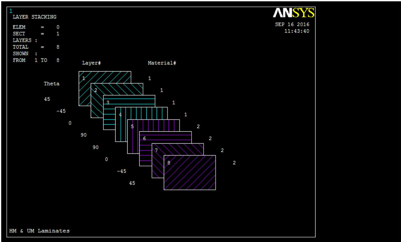
Figure 24. [(+/-45/0/90)<sub>s</sub>]<sub>n</sub> HM & UM Laminate Design Stacking Sequence.
