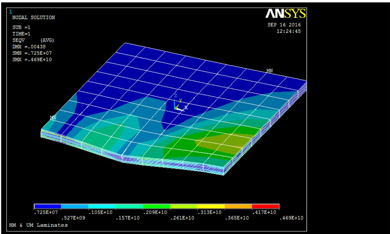
Figure 33. Von Mises Stress of HM & UM [(+/-45)s]<sub>n</sub> Laminate Design
