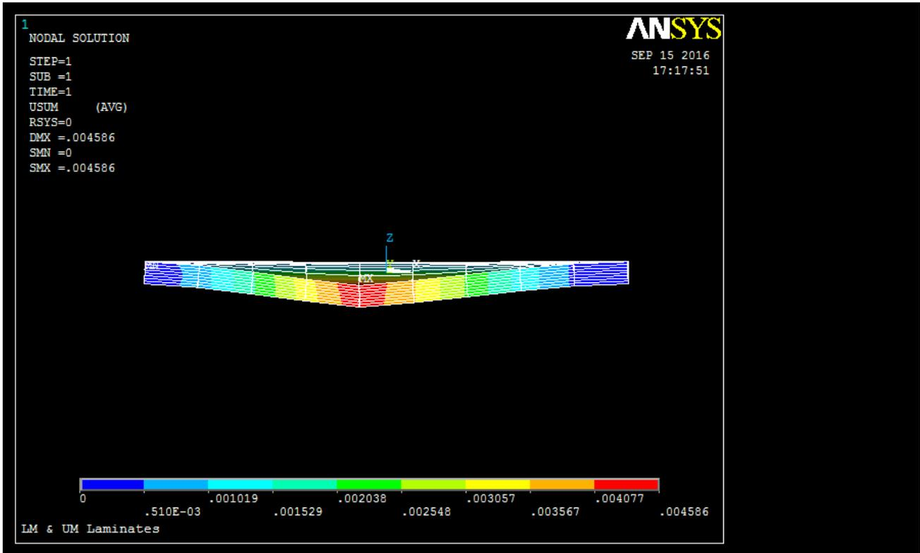
Figure 16. Deflection of LM & UM [(+/-45/0/90)s]<sub>n</sub> Laminate Design.
