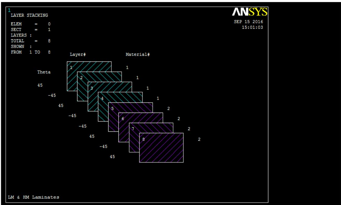
Figure 5. [(+/-45)<sub>s</sub>]<sub>n</sub> LM & HM Laminate Design Stacking Sequence
