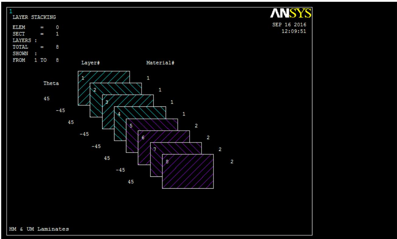
Figure 25. [(+/-45)<sub>s</sub>]<sub>n</sub> HM & UM Laminate Design Stacking Sequence.
