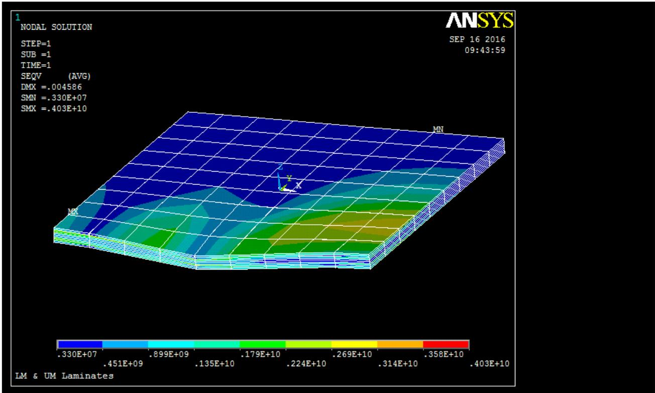
Figure 22. Von Mises Stress of LM & UM [(+/-45/0/90)s]<sub>n</sub> Laminate Design.
