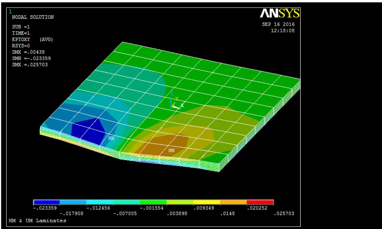
Figure 29. XY Shear Total Mechanical Strain of HM & UM [(+/-45)s]<sub>n</sub> Laminate Design.
