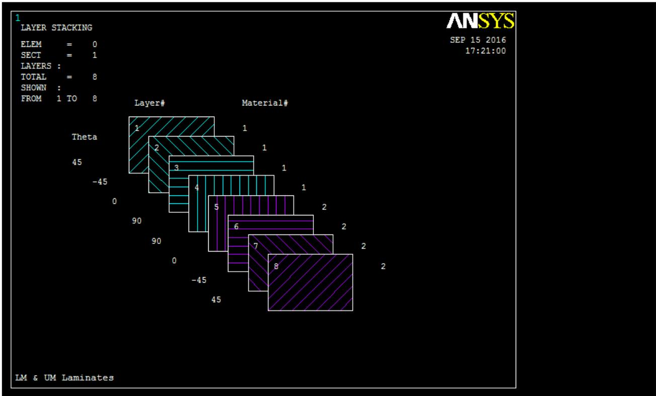
Figure 14. [(+/-45/0/90)<sub>s</sub>]<sub>n</sub> LM & UM Laminate Design Stacking Sequence.
