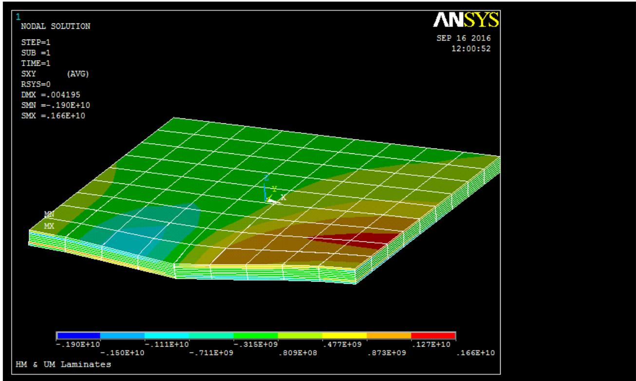
Figure 30. XY Shear Stress of HM & UM [(+/-45/0/90)s]n Laminate Design.
