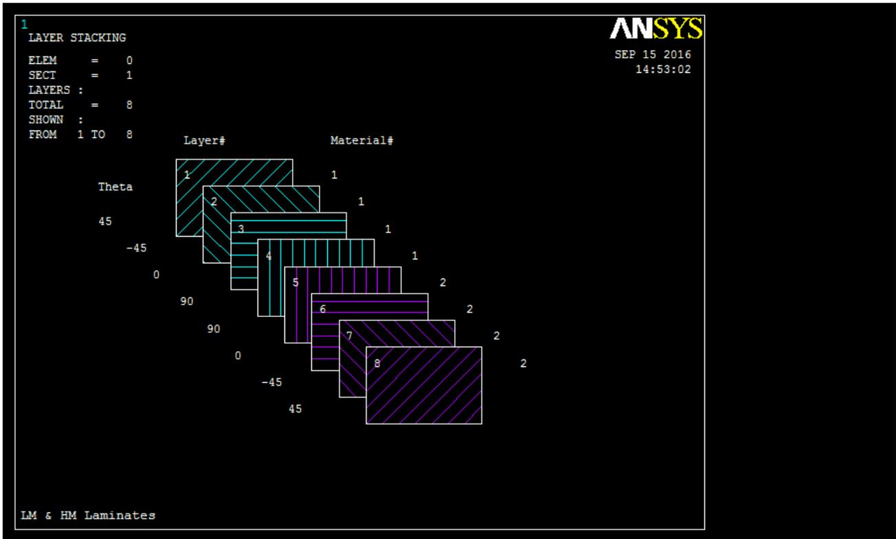
Figure 4. [(+/-45/0/90)<sub>s</sub>]<sub>n</sub> LM & HM Laminate Design Stacking Sequence
