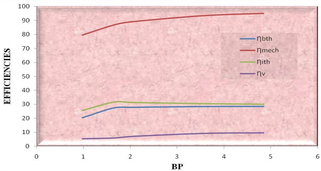
Graph 4. Variation of Brake Power (BP) with Efficiencies at 1300 rpm
