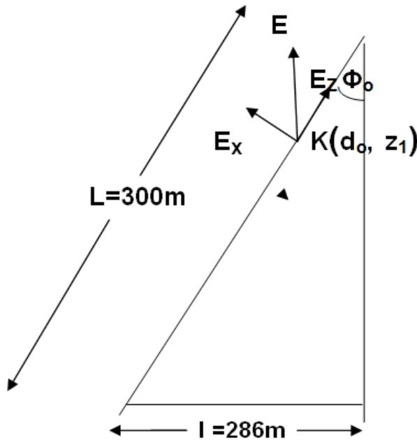
Figure 4. A lightning strikes the cable length L at the point K( $d_o, z_1$ ) and an electric field E is produced
