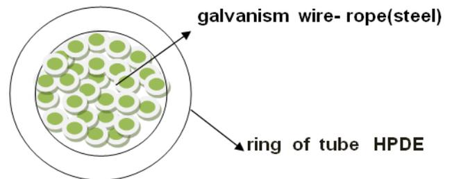
Figure 3. The cable is a composite material.
