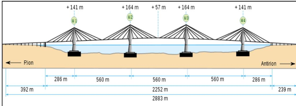
Figure 2. Schematic view of the Rion –Antirion bridge. Taken from [3]
