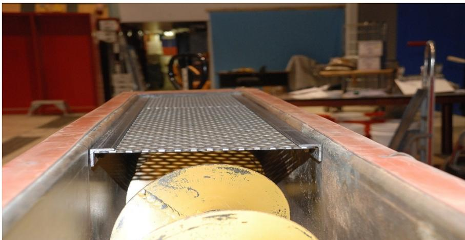
Figure 7. Fixed Grating Inside of Trough
