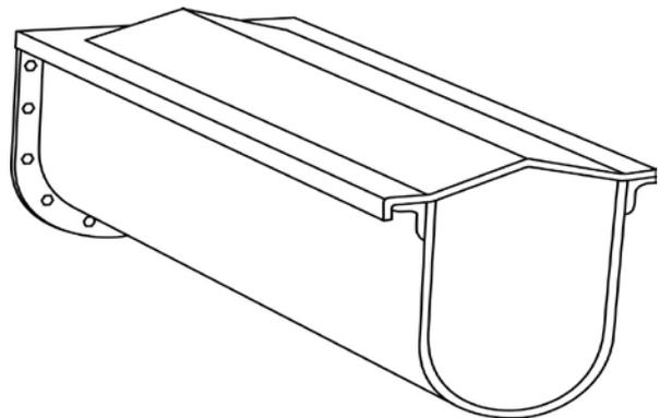
Figure 4b. Hip Roof Cover [ANSI/CEMA 350-1971, 2009 (After Figure 5.9D)]
