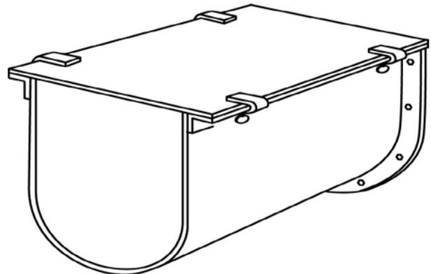
Figure 5a. Angle Flanged Type Trough With Plain Flat Cover Fastened with Thumb-Screw "C" Clamps [ANSI/CEMA 350-2009 (Figure 4. 16C)]
