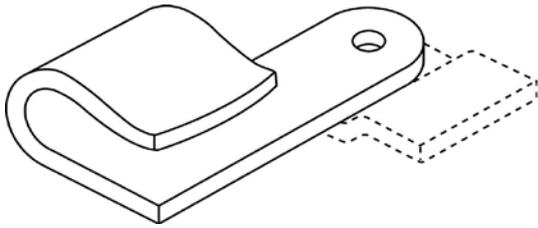
Figure 5d. Spring Cover Clamp Welding Bracket Optional
