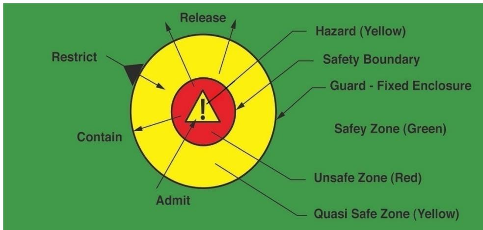
Figure 2. Operating Fixed Enclosure Guard
