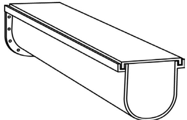
Figure 4c. Dust Seal Covers [ANSI/CEMA 350-1971, 2009 (After Figure 5.9B)]
