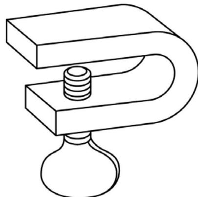
Figure 5c. Thumb-Screw Cover Clamp [ANSI/CEMA 350-2009 (Figure 4. 16E)]
