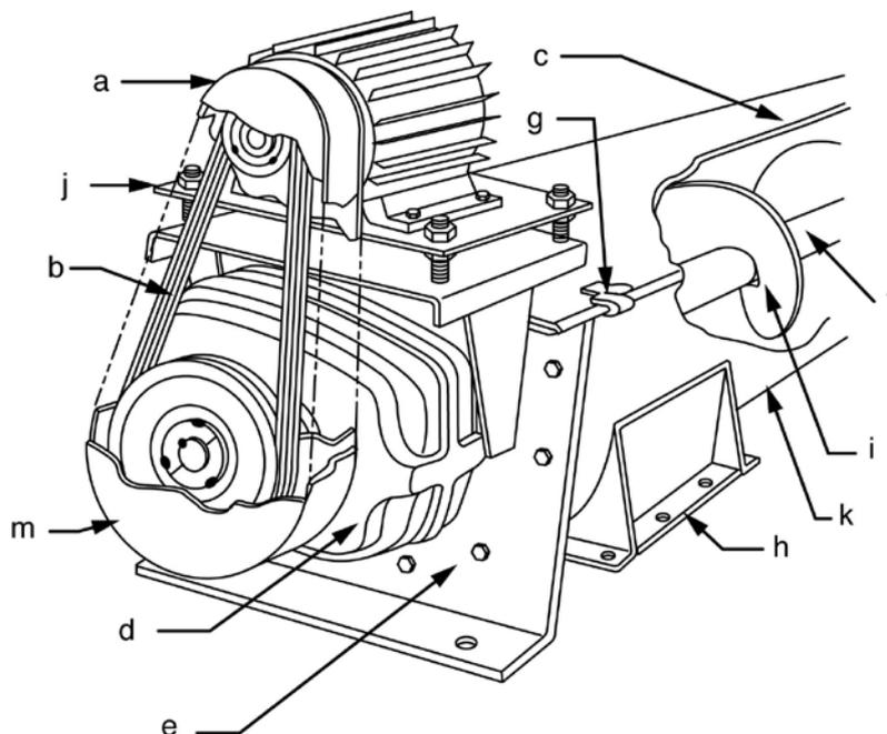
Figure 1. Typical Horizontal Screw Conveyor System [Taken from Figure 8.1, ANSI/CEMA 350-2009]
