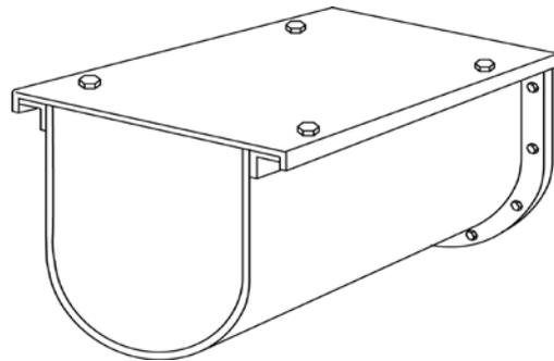
Figure 6. Angle Flanged Type Trough With Flanged and Bolted Cover [ANSI/CEMA 350-1971, 2009 (Figure 4.16A)]
