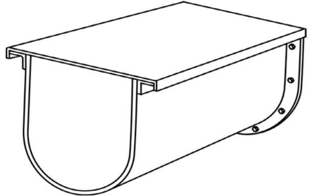
Figure 4a. Conventional Flanged Cover [ANSI/CEMA 350-1971, 2009 (After Figure 1.4)]
