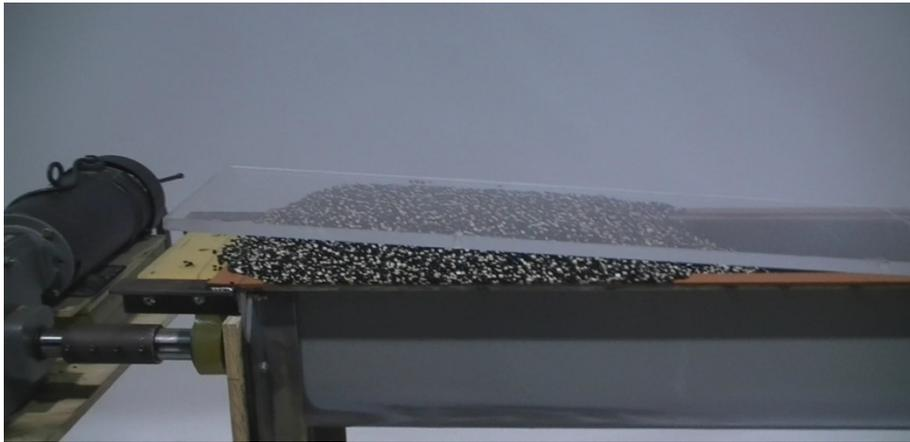
Figure 8. Material Driven to Dead End - Bulging Lifts Plastic Cover
