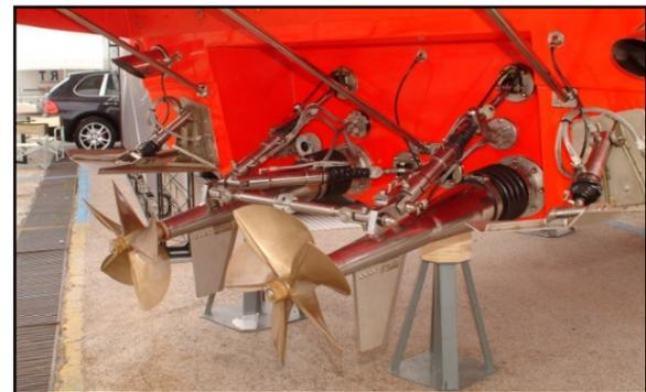
Figure 5. Top system Surface Drive
