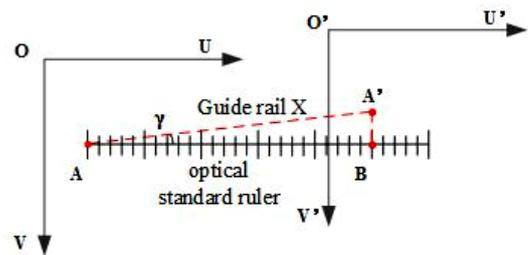
Figure 7. The diagram of measuring the inclination of the guide rail X
