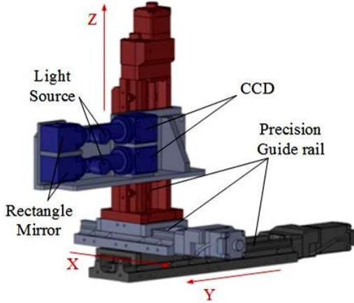
Figure 4. Vision alignment device
