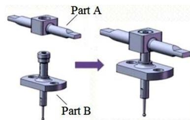
Figure 2. Assembly process of small interference fitting parts
