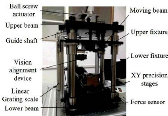
Figure 1. Precision press-fit instrument
