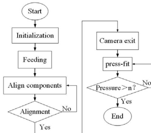
Figure 3. Flowchart for the assembly process of the precision press-fit instrument
