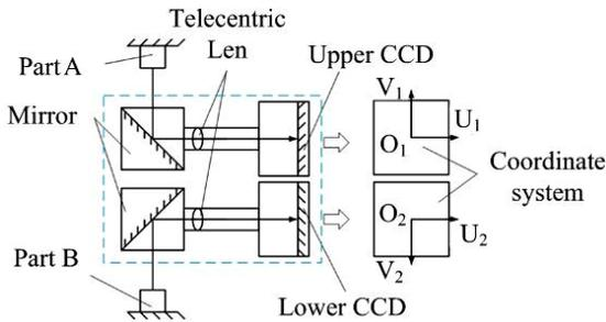
Figure 5. The structure diagram of the upper and lower cameras
