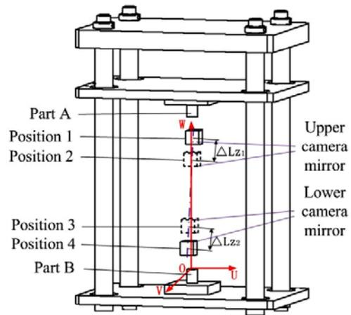
Figure 6. The error analysis diagram of guide rail Z
