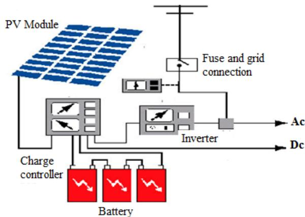
Figure 1. Configurations of PV system
