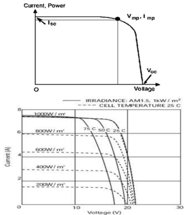
Figure 4. PV Voltage current characteristic curves
