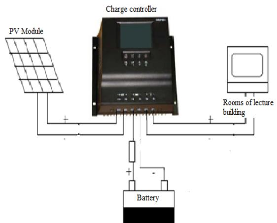
Figure 7. Charge controller system configuration.
