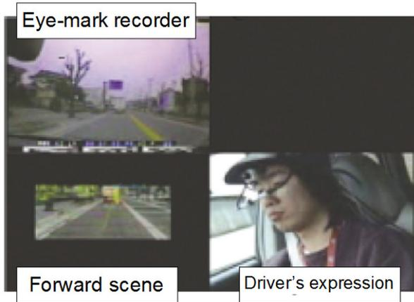
**Figure 4.** Picture of the experimental situation. The upper-left picture shows the field view from the eye-mark recorder, lower-left picture is the front scene from a stereo camera, and lower right is the face of a subject
