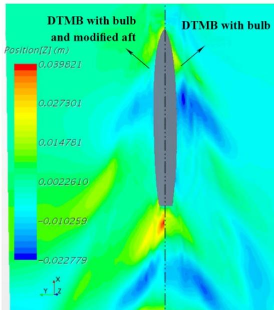
Figure 12. Wave pattern around the hull
