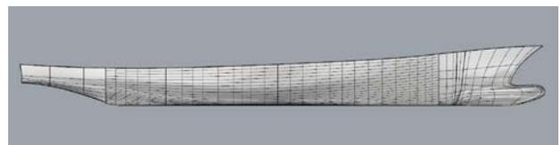
Figure 10. Bow and aft modification
