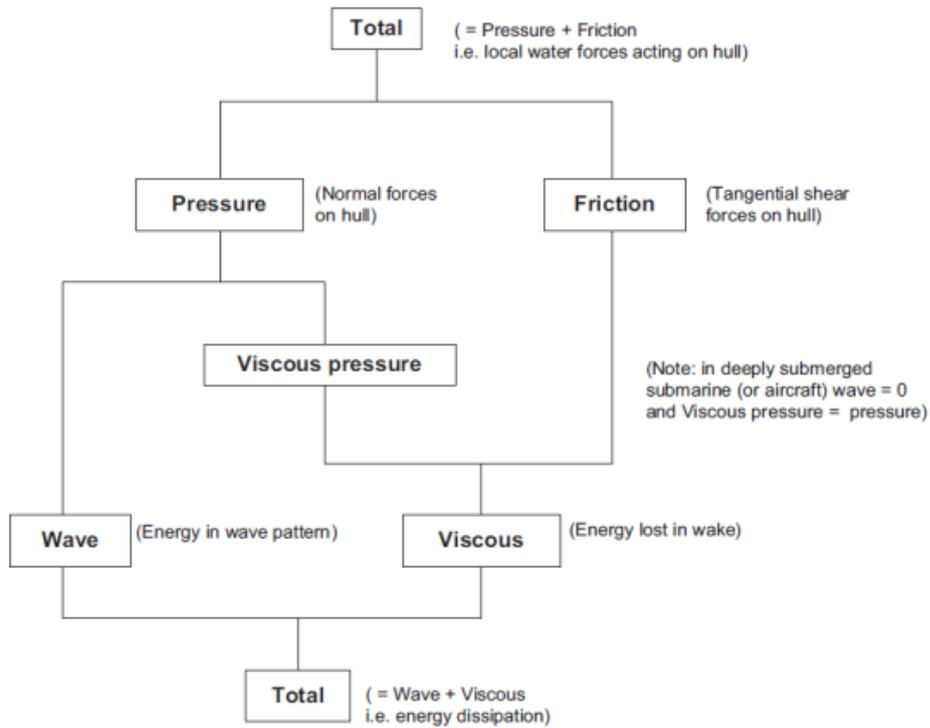
Figure 1. Basic resistance components
