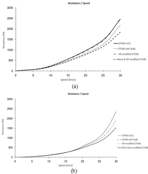
Figure 11. Aft and bow modification total drag (a) CFD (b) Maxsurf
