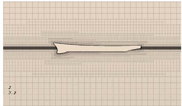
Figure 5. Mesh scene on free surface
