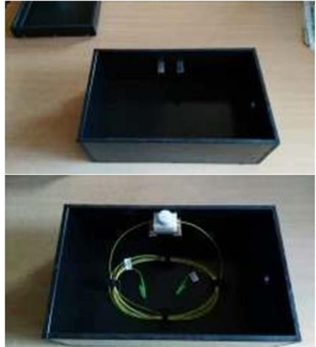
Figure 5. Placement of the sensor in the model of access chamber
