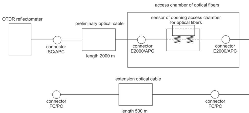
Figure 6. Schema of testing optical route
