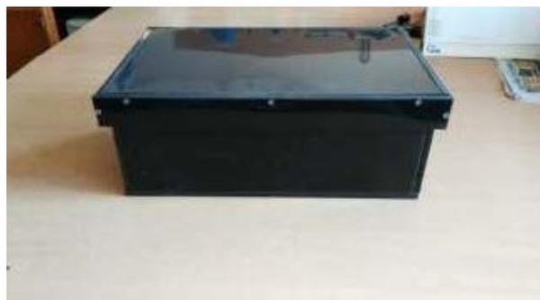
Figure 2. The plastic model of the access chamber for optical fibers
