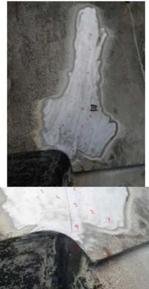
Figure 13. Points of hardness measurement in area III – crack neighborhood
