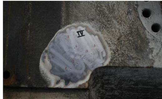
Figure 14. Points of hardness measurement in area IV
