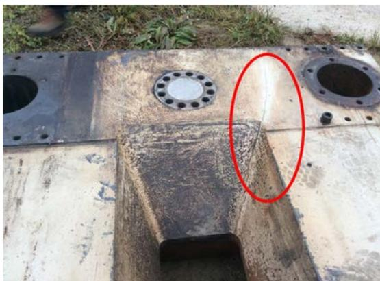
Figure 6. Stationary plate with a crack
