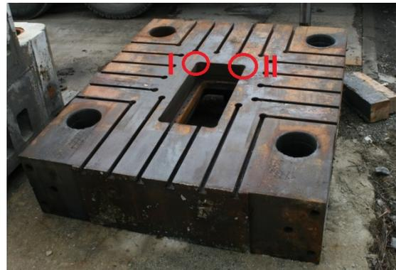
Figure 7. Areas of hardness measurement from the side of the casting mold (I and II)
