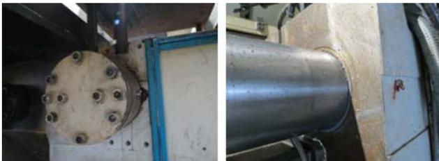
Figure 5. Fixing the nut of the guide column to the stationary section
