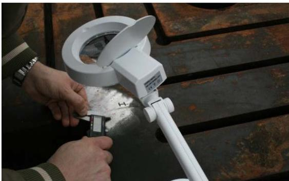
Figure 11. Reading of the indentation diameter on the tested plate (area I, point 5) using a digital gauge and a magnifier
