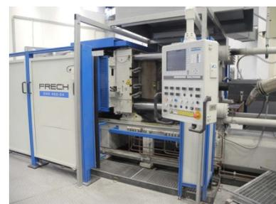
Figure 3. Die casting machine [2]
