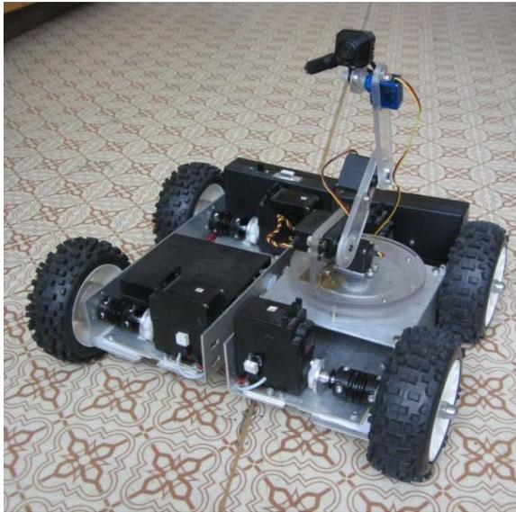
**Figure 2.** Chassis frame of mobile robot
