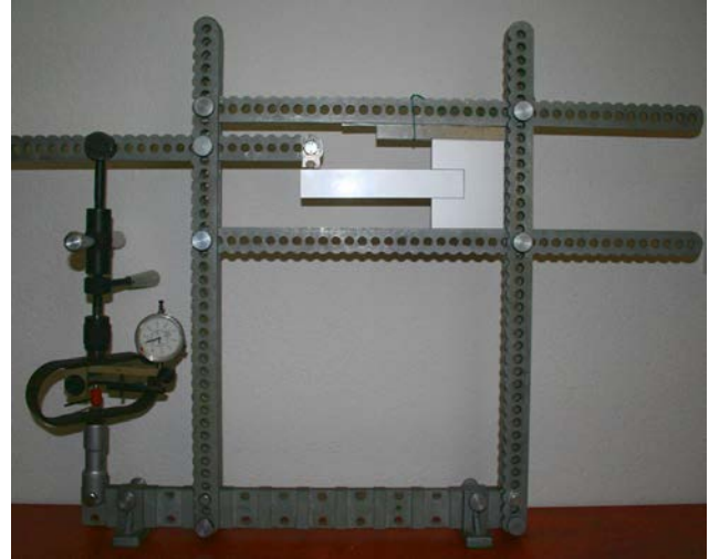
Figure 3. Specimen located in the loading system with a lever mechanism
