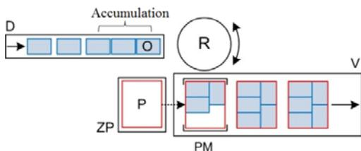
Figure 6. Structure workplace with accumulative conveyor - during pallet changes
