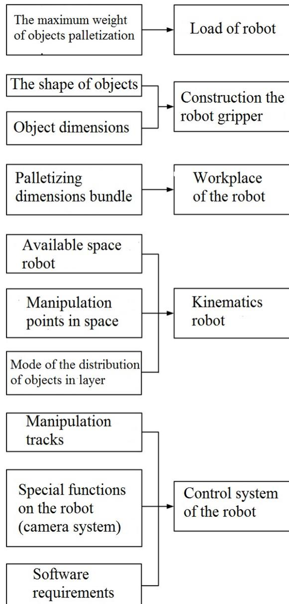
Figure 2. Decisive criteria for selection of palletizing robot
