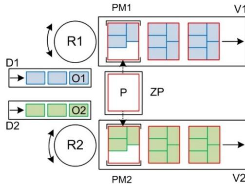
Figure 8. The structure workplace with two robots - more types of objects, a common stack of empty pallets
