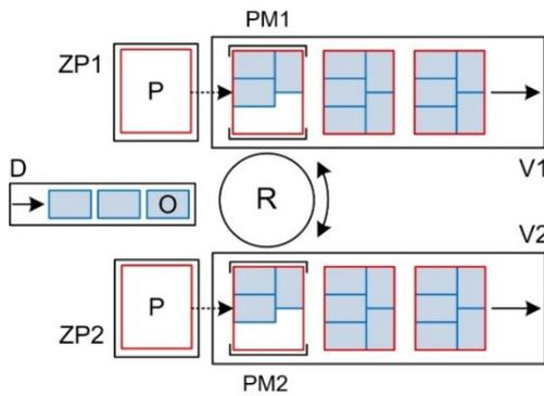
Legend: It is not time for reserve to change palettes (i.e. ZP1 from stack moves the pallet PM1 and in the meantime it is possible to handle objects palletizing PM2). During the palletizing PM2 is realized by reloading pallets for PM1 in an overlapping time.
