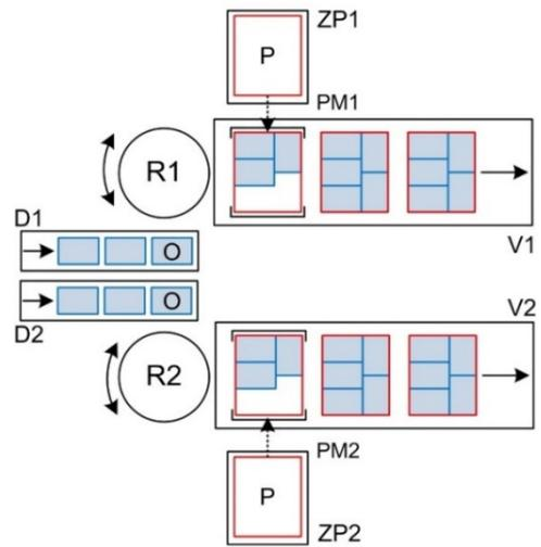
Figure 7. Structure workplace with two robots - one type of object
