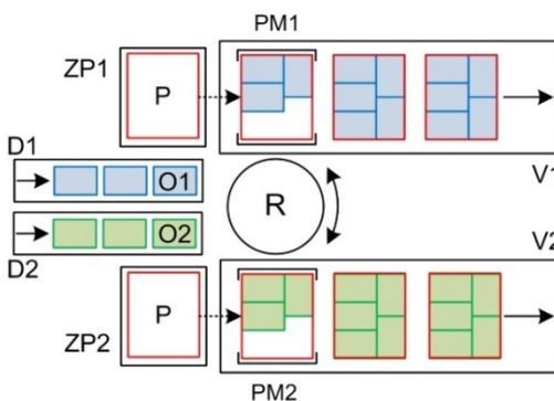
Figure 5. Structure workplace with two place of palletizing - palletizing of two different kinds of objects
