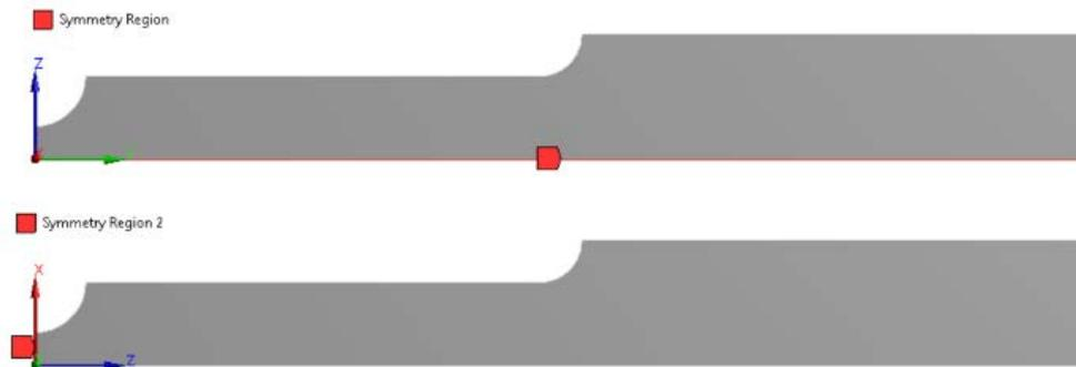
Figure 10. Defined symmetry regions in numerical model created in Ansys Workbench
