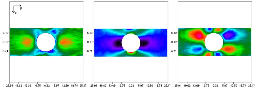
Figure 3. Illustrative strain fields obtained from Q-300 Dantec Dynamics
