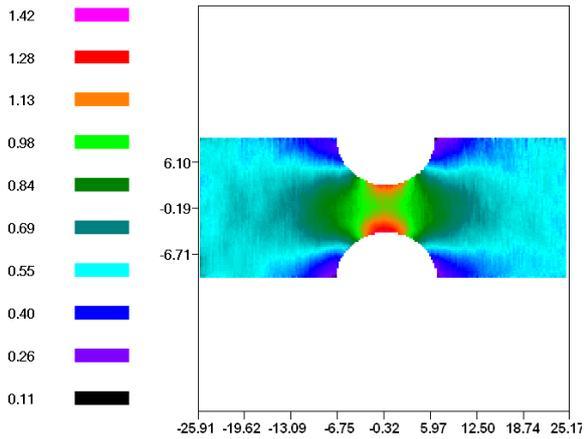
Figure 9.  $\epsilon_y$  [mm/m] strain field acquired by loading force of 1700 N
