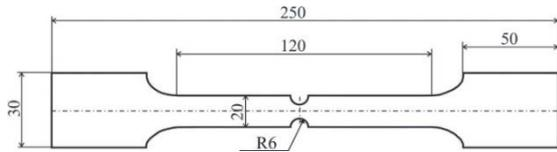
Figure 4. Shape and dimensions of the specimen
