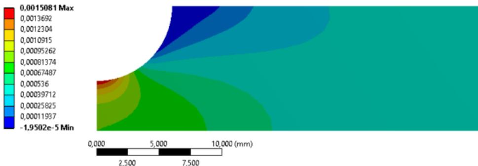
Figure 12.  $\epsilon_y$  strain field acquired numerically by maximal loading force
