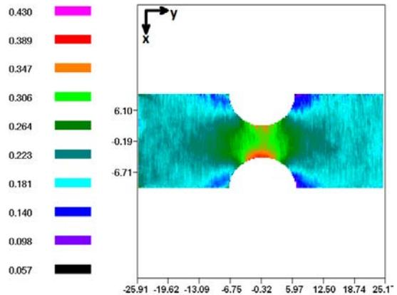
Figure 6.  $\epsilon_y$  [mm/m] strain field acquired by loading force of 450 N
