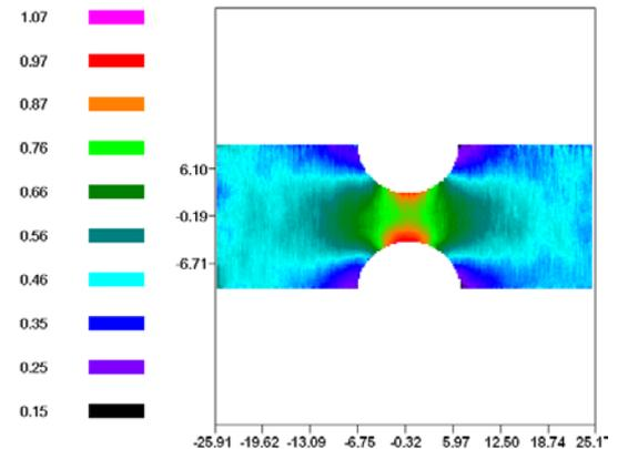
Figure 8.  $\epsilon_y$  [mm/m] strain field acquired by loading force of 1250 N
