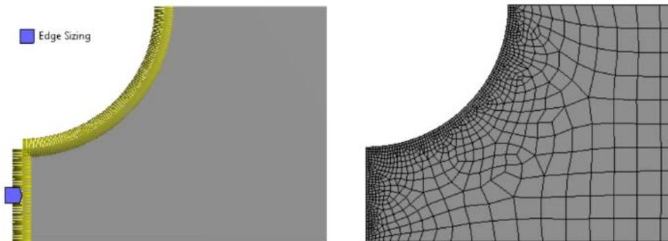
Figure 11. Resizing of the mesh in the area of notch
