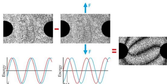
Figure 1. Speckle effect for unloaded and loaded state with the results of subtraction
