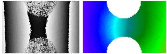
Figure 2. Typical  $2\pi$  phase image (left) and corresponding phase map (right)
