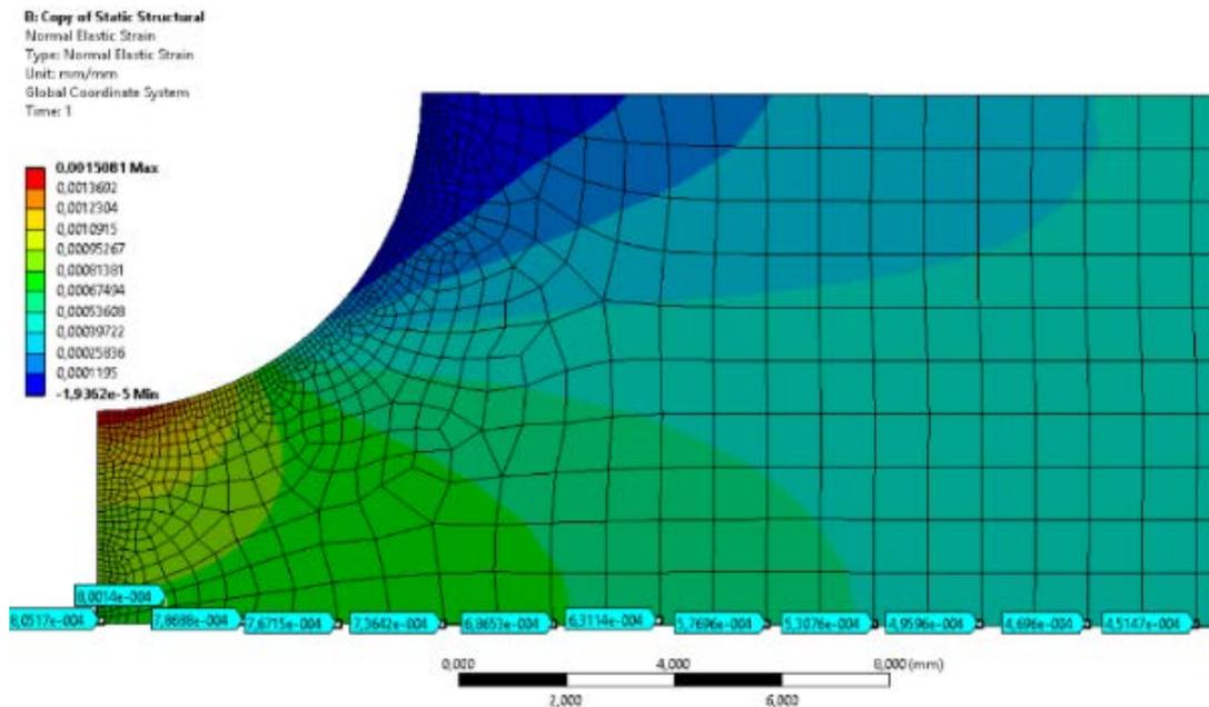
Figure 14. A half of overall amount of virtual gages used in Ansys Workbench
