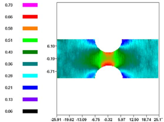
Figure 7.  $\epsilon_y$  [mm/m] strain field acquired by loading force of 850 N
