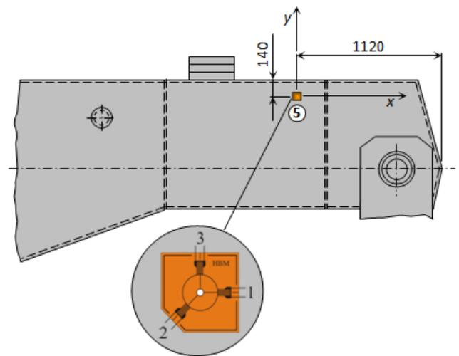
Figure 4. Strain gauge in position 5
