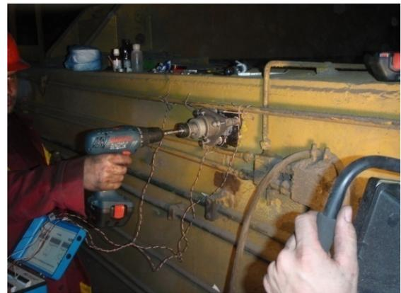
Figure 3. Hole drilling in position 5 on the transversal beam
