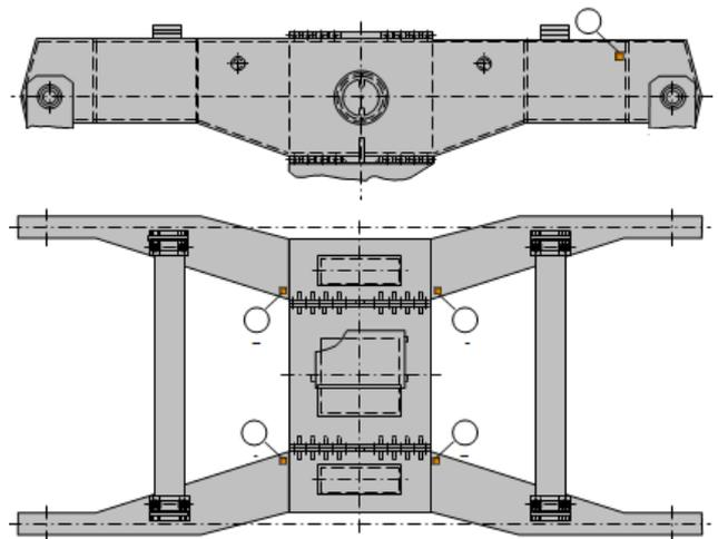
Figure 2. Strain gauge mounting positions on the transversal beam
