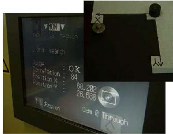
Figure 4. Recognition and assignment of X and Y coordinates for object
