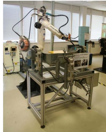
Figure 5. Robotized workplace with industrial robot ALMEGA AX-V6
