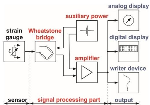
Figure 2. Scheme of measurement chain for the measurement of deformations by strain gages
