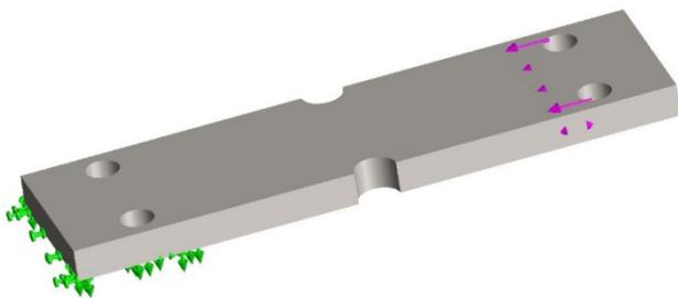
Figure 10. Model of analyzed specimen with boundary conditions
