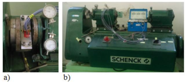
Figure 8. Loading equipment SCHENCK. a) location of test specimen in working space, b) view to measurement chain
