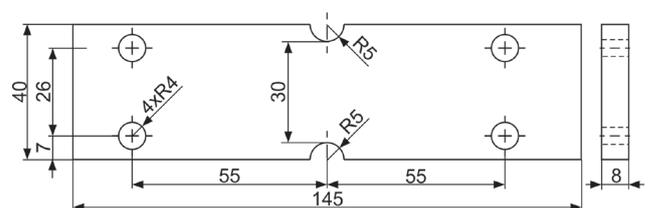
Figure 1. Dimensions and shape of test specimen
