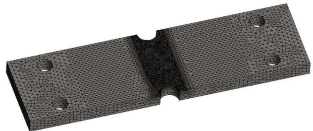
Figure 12. Meshed model with refined mesh near stress concentrators
