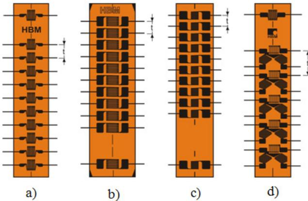
Figure 4. Shapes of strain gage chains. a) direction of measurement grid is parallel with longitudinal axis of chain, b) direction of measurement grid is perpendicular to longitudinal axis of chain, c) direction of measurement grid is oriented parallel or perpendicular to longitudinal axis of chain, d) measurement grids are in groups with three and angles 0°/60°/120° with respect to longitudinal axis of chain [8]
