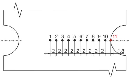
Figure 11. Numbering of sensors on analyzed model
