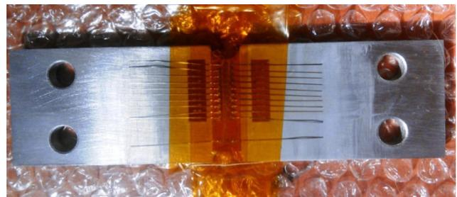
Figure 6. Position of strain gage chain
