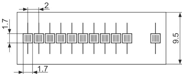
Figure 5. Basic dimensions of strain gage chain KY21-2/120 [8]
