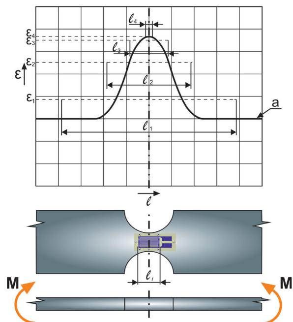
Figure 3. Influence of grid length  $\ell_i$  to the measured value of strain
