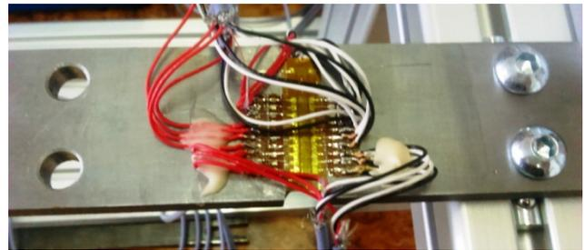
Figure 7. View to applied strain gage chain with soldered wires
