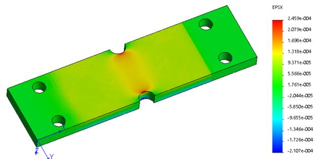
Figure 13. Strain field  $\epsilon_x$  for defined loading
