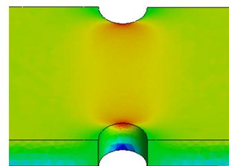
Figure 14. Detail of strain field  $\epsilon_x$  near analyzed notches
