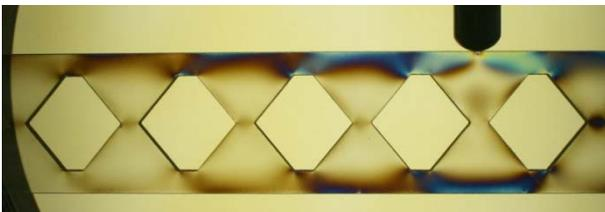
**Figure 17.** Field of isochromatics around analyzed concentrators – variant B
