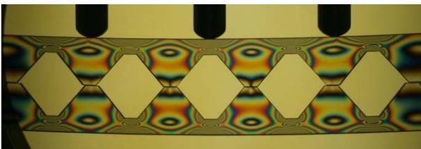
**Figure 18.** Field of isochromatics around analyzed concentrators – variant C
