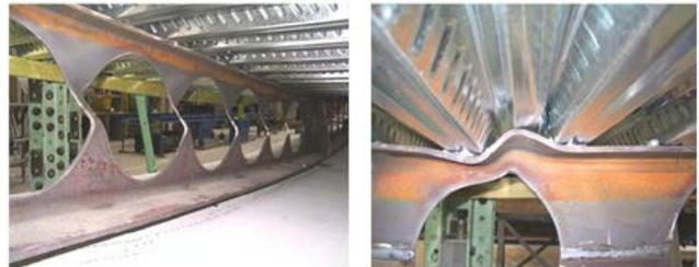
**Figure 20.** Collapsed cellular beam [11]
