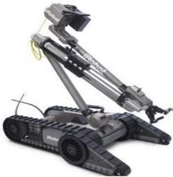
Figure 1. Little pyrotechnic robot iRobot
