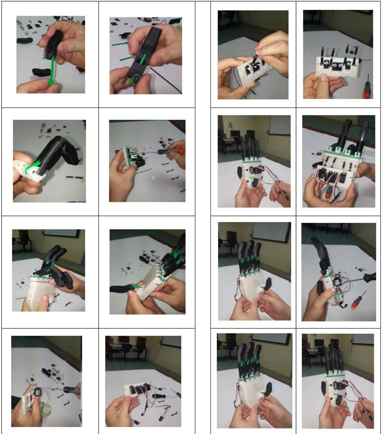
Figure 10. assembly robotic hand
