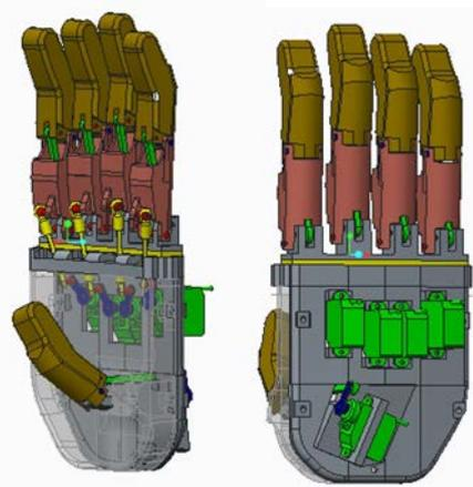
Figure 1. Variant prototype robotic hand right
