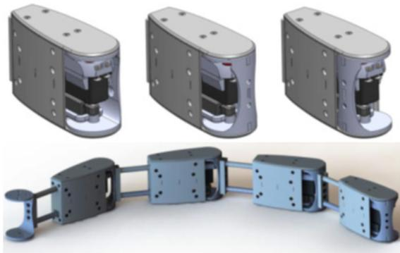
**Figure 1.** 3D model of LocoSnake link a) +90° b) 0° c) -90° d) 50 (mm) protrusion of every segments
