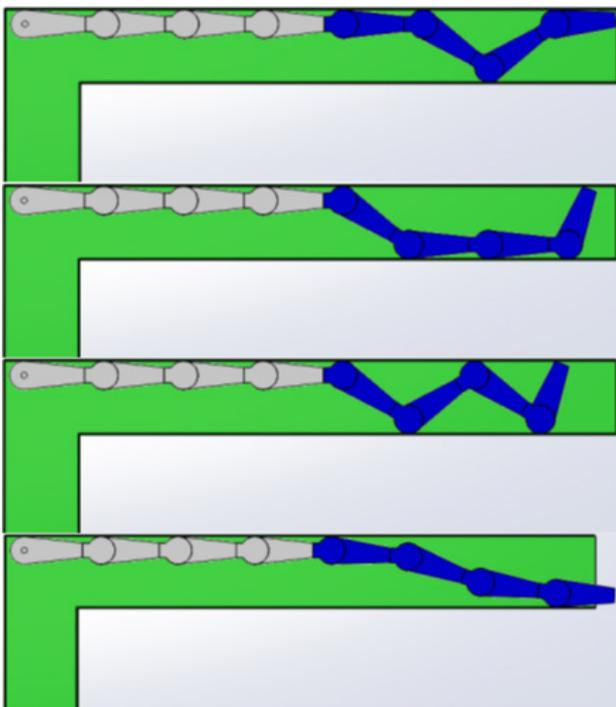
Figure 6. Fixation curves applied on LocoSnake
