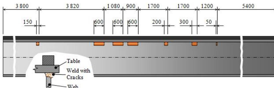
Figure 2. Length of cracks on beam structure
