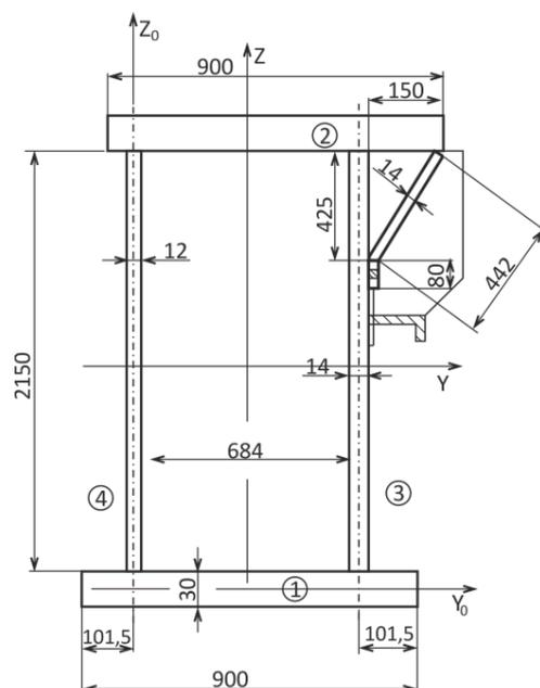
Figure 4. Alteration of the main beams cross section
