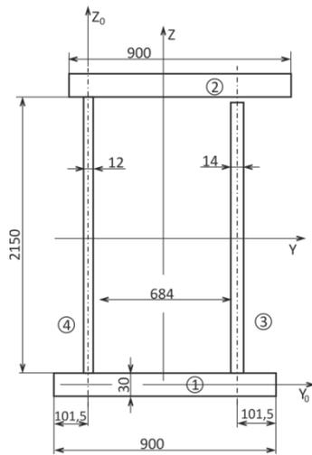
Figure 3. Open profile of the main beam
