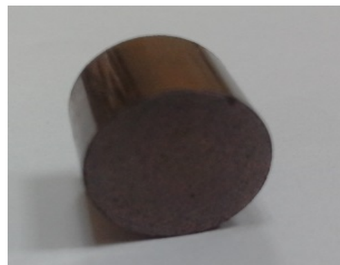
Figure 2. Additive mixed Cu-W P/M composite electrode
