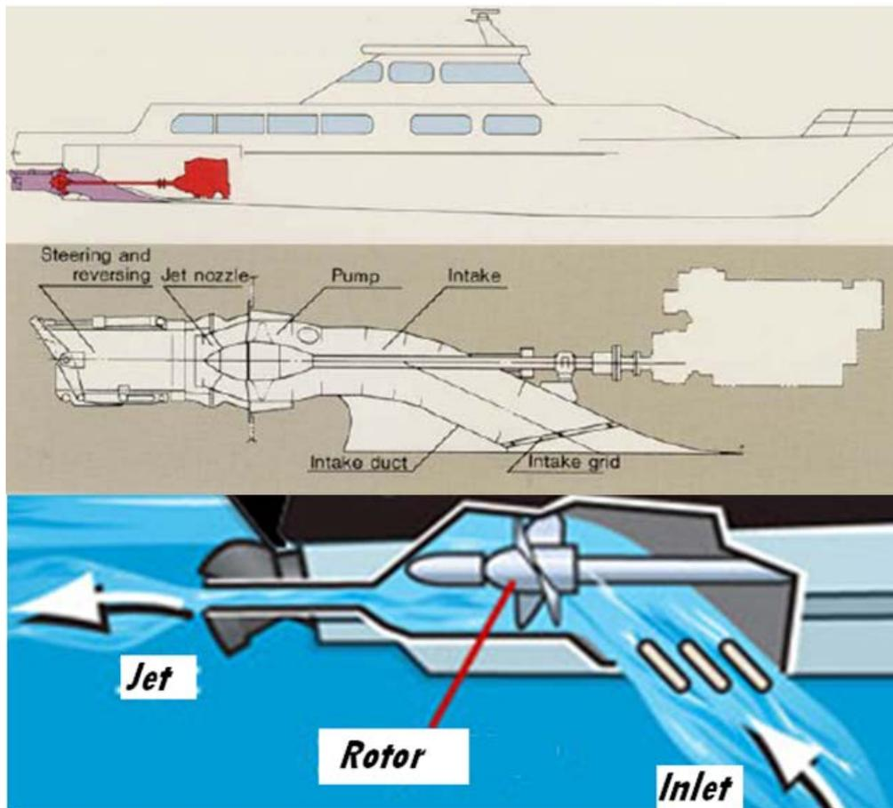
Figure 1. Schematic of the system
