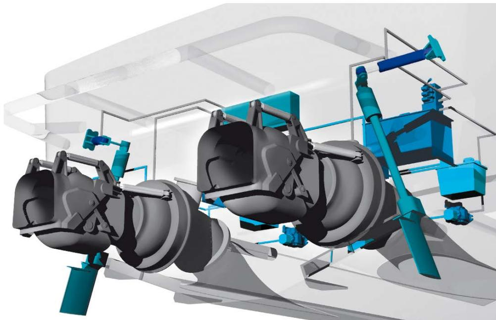
Figure 2. Schematic of the twin-waterjet system
