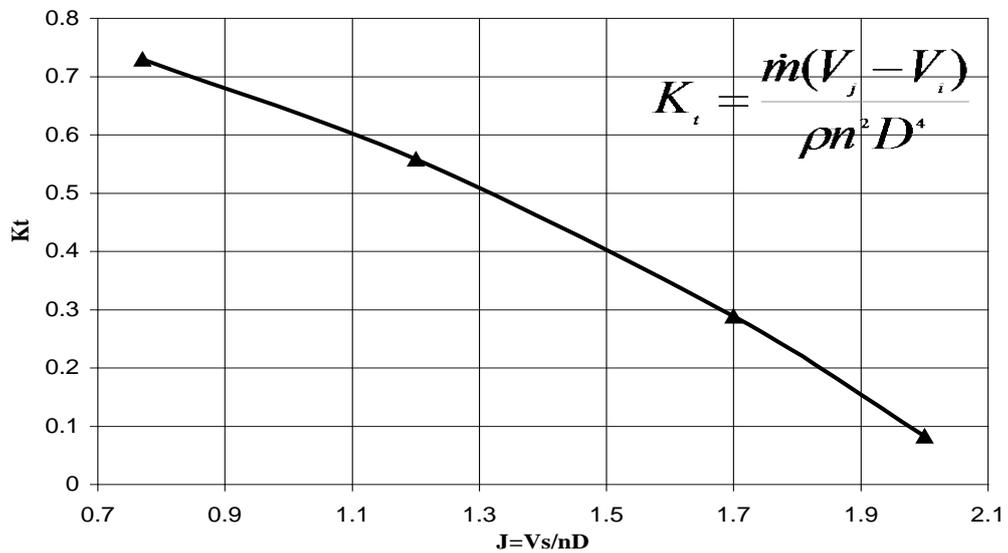
Figure 6. Thrust coefficient at various speeds
