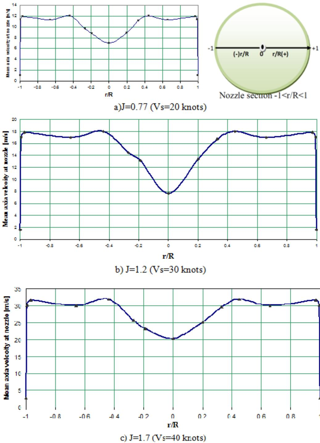
Figure 8. Axial velocity at nozzle at different velocities
