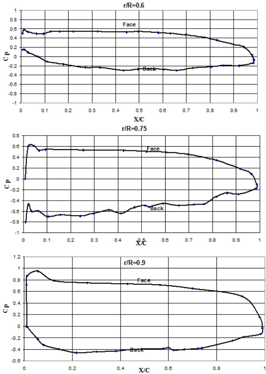
Figure 5. Pressure distribution on rotor blade at  $J=1.7$
