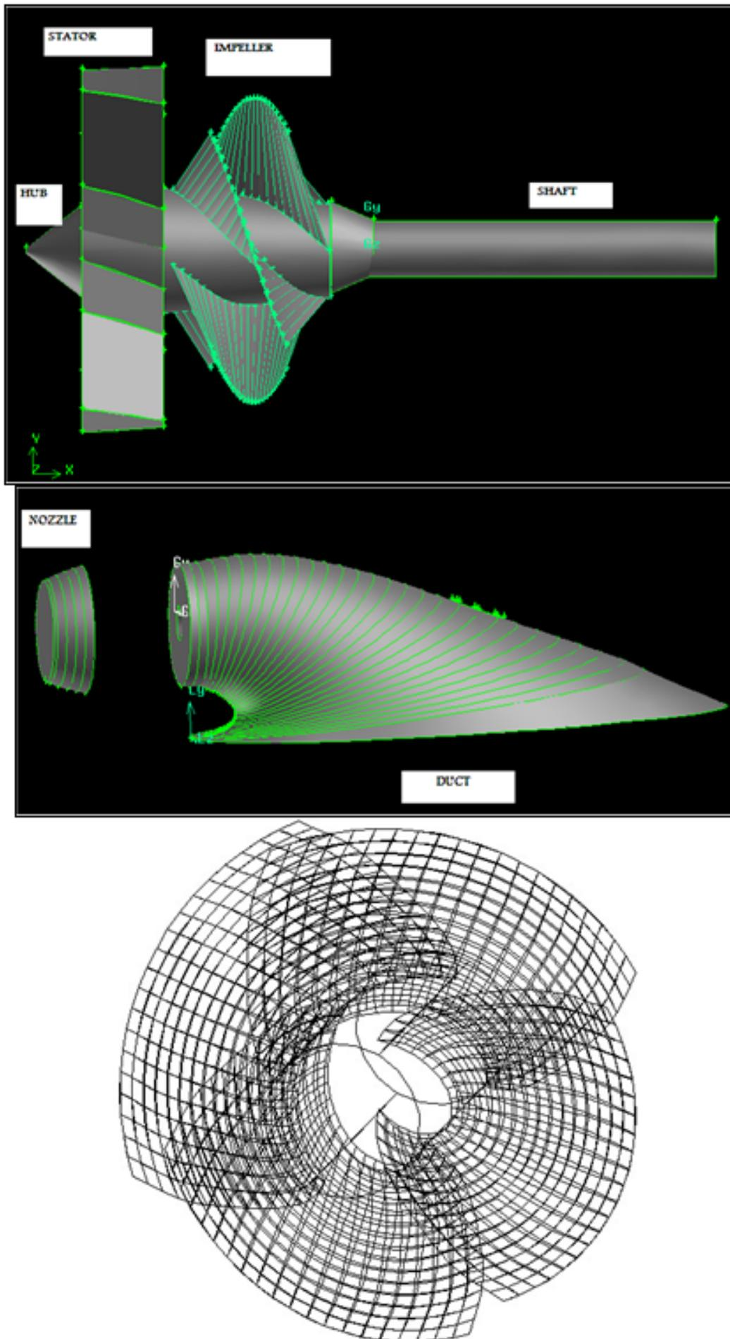
Figure 4. View showing rotor, duct and stator
