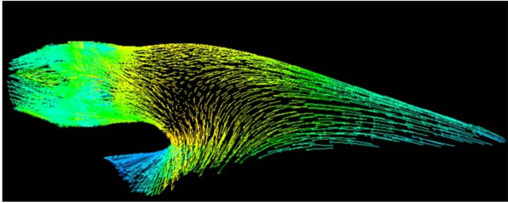
Figure 7. Flow velocity vector on the duct at  $J=1.7$
