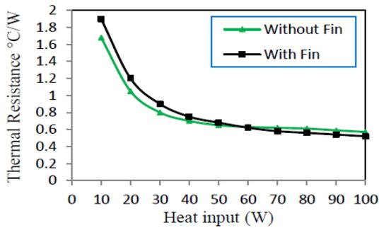
Figure 13. Variation of thermal resistance with heat input for different structures with acetone at 70% filling ratio and 0° inclination angle
