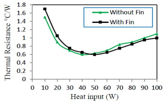
Figure 12. Variation of thermal resistance with heat input for different structures with acetone at 40% filling ratio and 0° inclination angle
