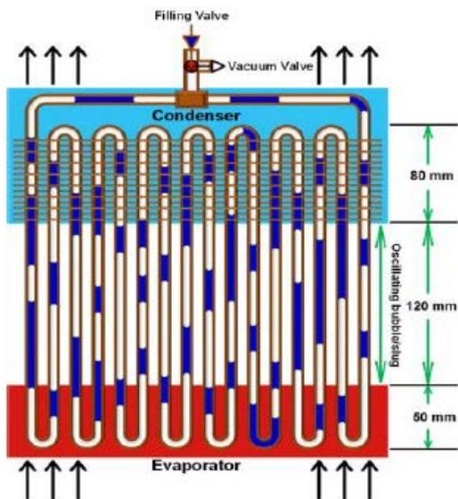
Figure 2. CLPHP with fin Structure
