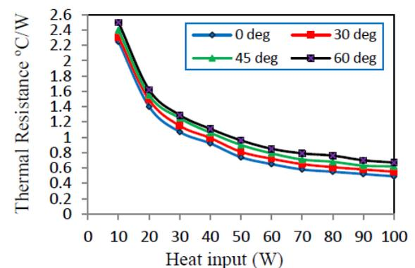
Figure 7. Variation of thermal resistance with heat input at different inclination angle with 50% filling ratio
