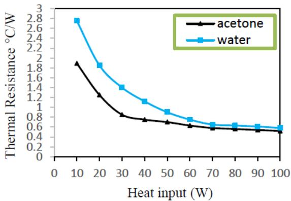
Figure 8. Variation of thermal resistance with heat input at 70% filling ratio and 0° inclination angle
