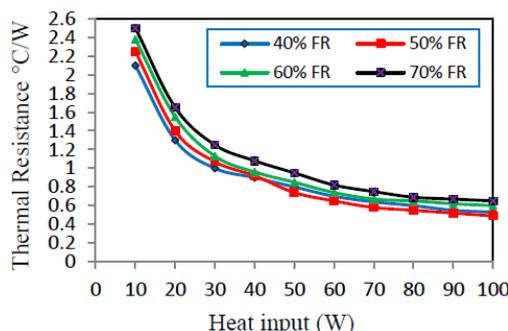
Figure 5. Variation of thermal resistance with heat input for different filling ratio at 0° inclination angle
