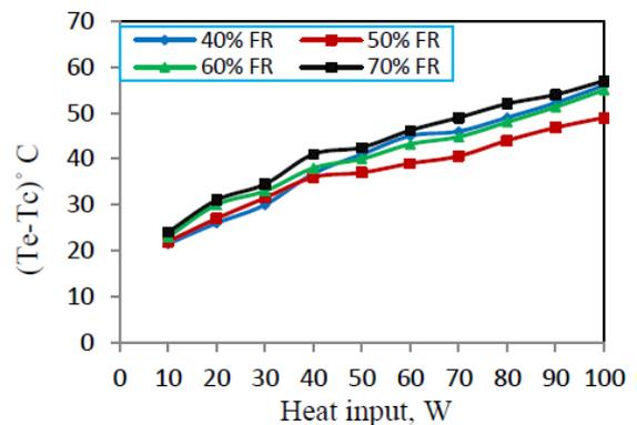
Figure 17. Variation of temperature difference between evaporator and condenser section with heat input for different working fluids at 0° inclination
