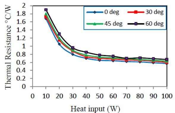
Figure 6. Variation of thermal resistance with heat input at different inclination angle with 70% filling ratio
