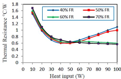
Figure 4. Variation of thermal resistance with heat input for different filling ratio at 0° inclination angle
