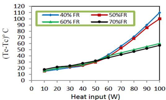
Figure 15. Variation of temperature difference between evaporator and condenser section with heat input for different working fluids at 0° inclination
