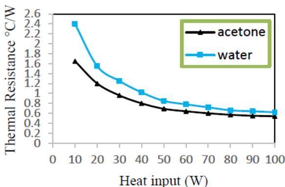
Figure 10. Variation of thermal resistance with heat input at 70% filling ratio and 0° inclination angle
