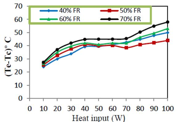
Figure 18. Variation of temperature difference between evaporator and condenser section with heat input for different working fluids at 0° inclination
