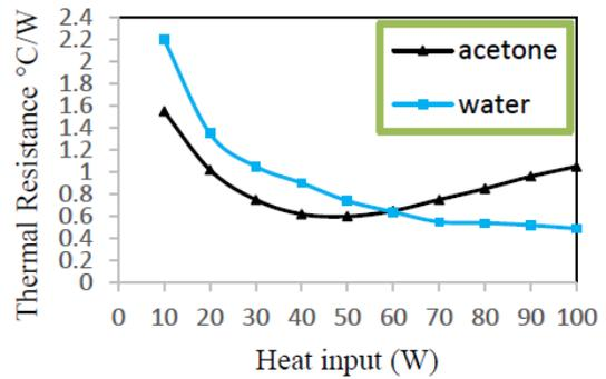
Figure 11. Variation of thermal resistance with heat input at 50% filling ratio and 0° inclination angle
