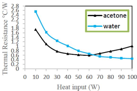
Figure 9. Variation of thermal resistance with heat input at 50% filling ratio and 0° inclination angle
