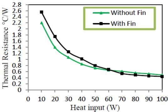
Figure 14. Variation of thermal resistance with heat input for different structures with acetone at 50% filling ratio and 0° inclination angle
