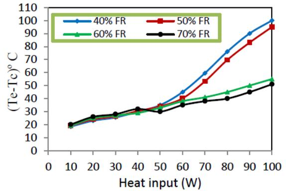
Figure 16. Variation of temperature difference between evaporator and condenser section with heat input for different working fluids at 0° inclination
