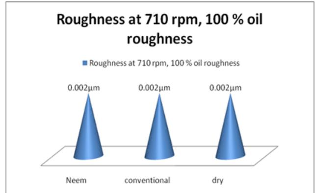
**Figure 18.** Plot of average surface roughness at 100% oil, 710 rpm, 0.5 mm depth of cut and dry sample
