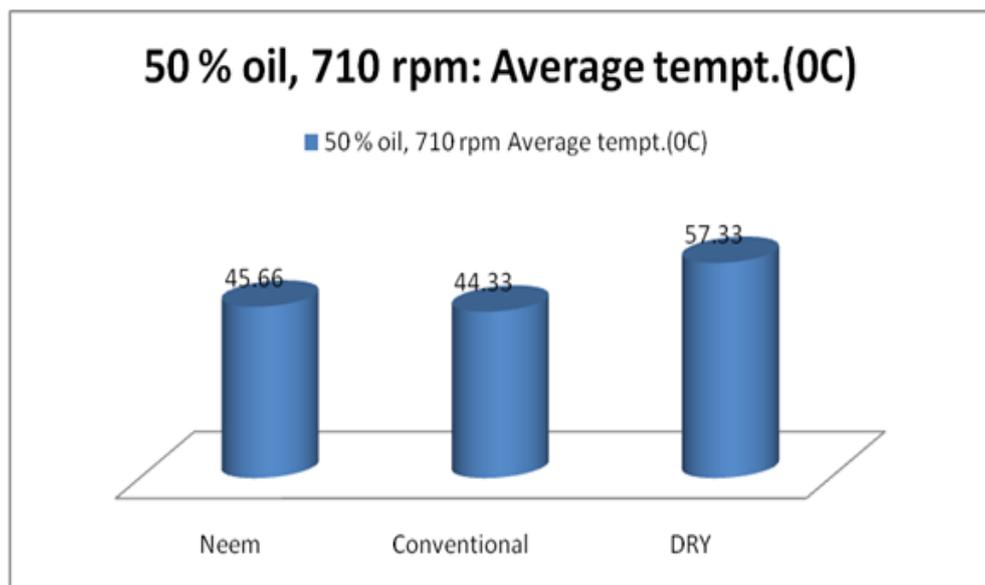
**Figure 7.** Average Temperatures (°C) of samples machined with 50% oil/50% water ratio and dry sample, 710rpm, 0.5mm depth of cut
