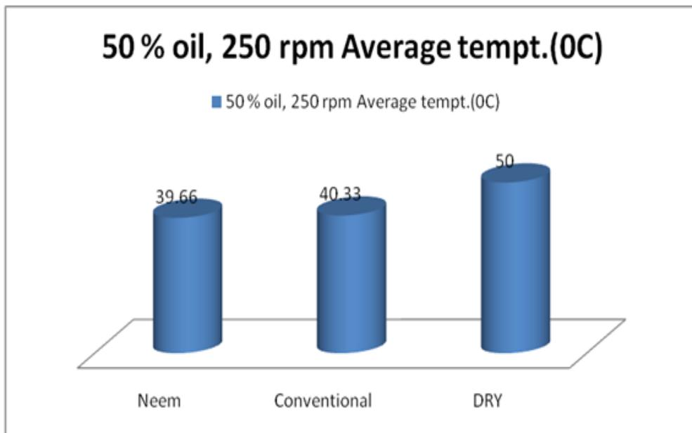
**Figure 6.** Average Temperatures (°C) of samples machined with 50% oil/50% water emulsion ratios and dry sample, 250 rpm, 1 mm depth of cut
