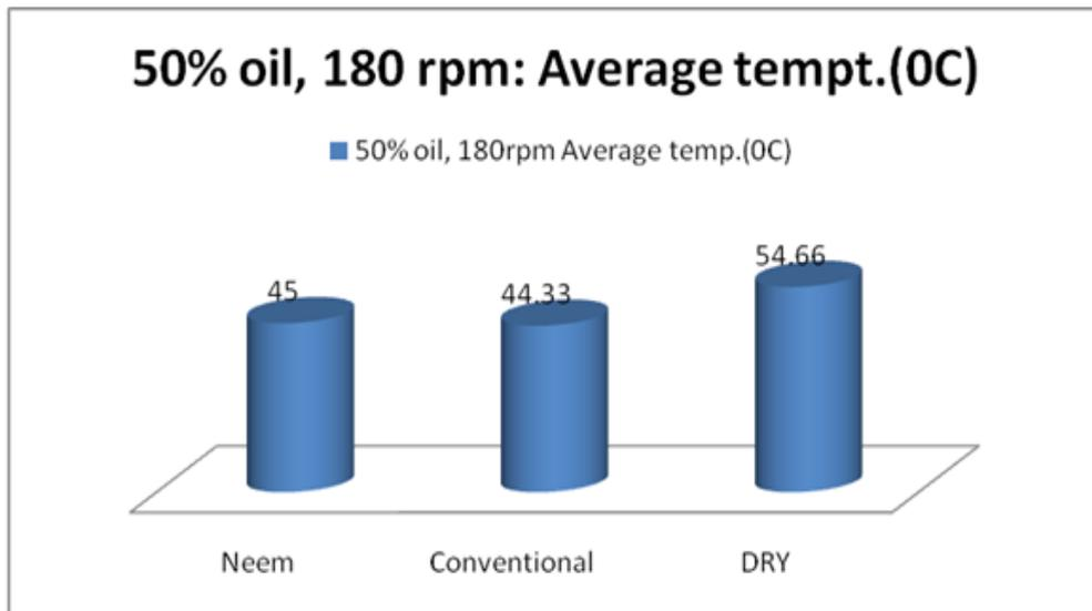
**Figure 5.** Average Temperatures (°C) samples machined with 50% oil/50% water ratio and dry sample, 180rpm, 0.75mm depth of cut
