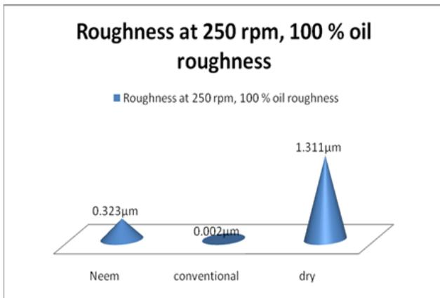
**Figure 15.** Plot of average surface roughness at 100 % oil, 250 rpm, 1mm depth of cut and dry sample
