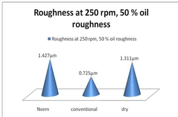
**Figure 16.** Plot of average surface roughness at 50 % oil, 250 rpm, 1mm depth of cut and dry sample
