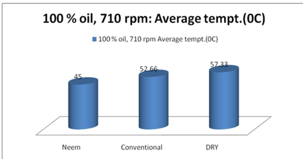
Figure 4. Average Temperatures (°C) of samples machined with 100% straight oils and dry sample, 710rpm, 0.5mm depth of cut
