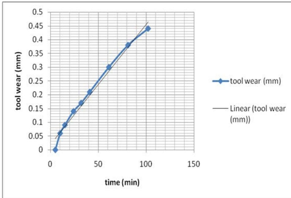
Figure 11. Plot of tool wear (mm) versus machining time (min) of HSS (12 X 200 mm) cutting tool
