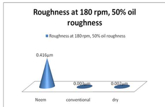
Figure 13. Plot of average roughness at 50 % oil, 180 rpm and 0.75 mm depth of cut
