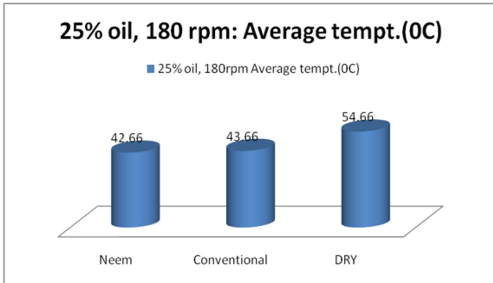
**Figure 8.** Average Temperatures (°C) of samples machined with 25% oil/75% water ratio and dry sample, 180rpm, 0.75mm depth of cut
