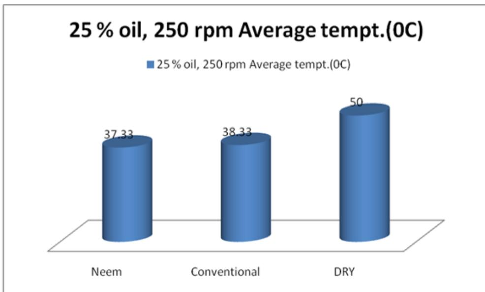
**Figure 9.** Average Temperatures (°C) of samples machined with 25% oil/75% water ratio and dry sample, 250rpm, 1mm depth of cut
