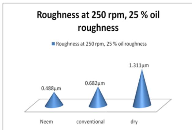
**Figure 17.** Plot of average surface roughness at 25 % oil, 250 rpm, 1 mm depth of cut and dry sample
