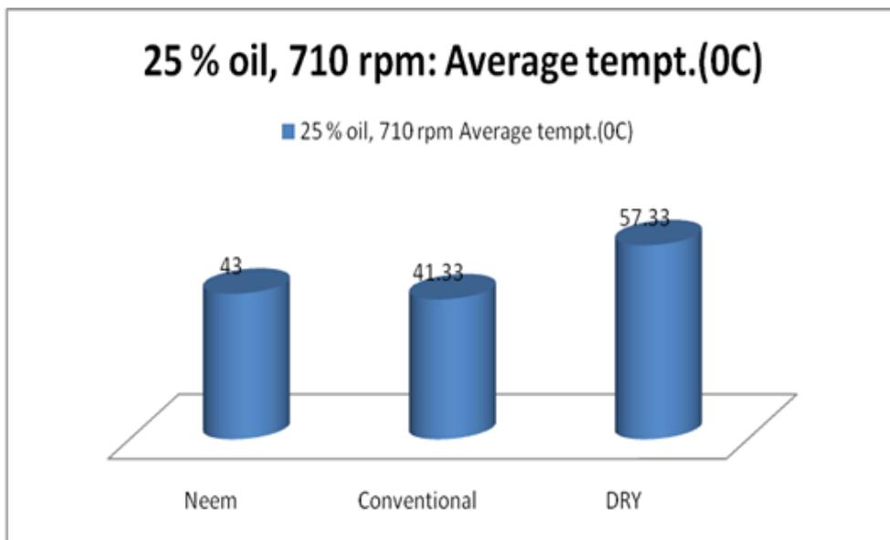
**Figure 10.** Average Temperatures (°C) of samples machined with 25% oil/75% water ratio and dry sample, 710rpm, 0.5mm depth of cut
