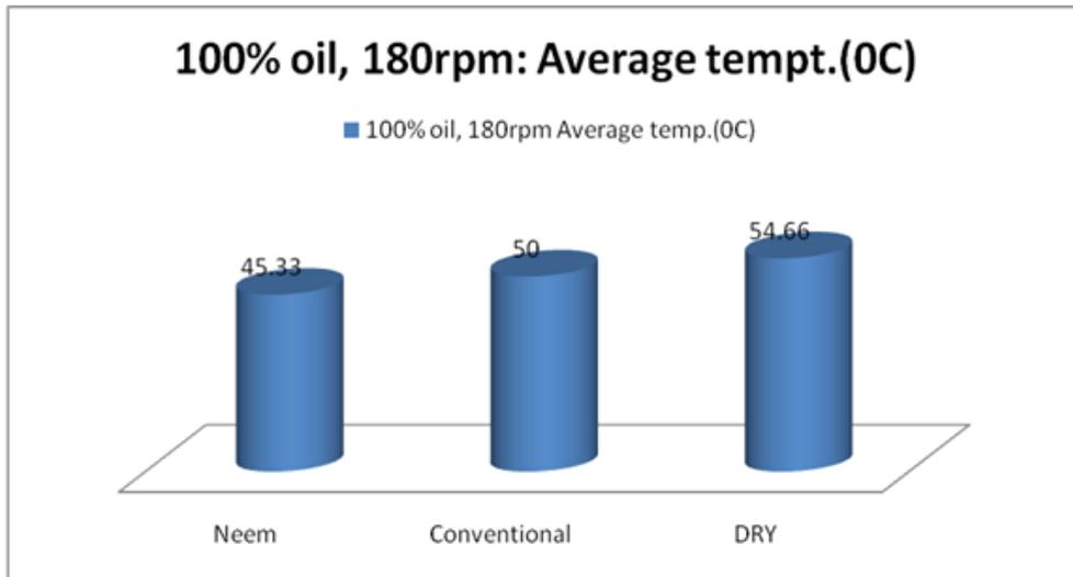
Figure 2. Average temperatures (°C) of samples machined with 100% straight oil and dry sample, 180rpm, 0.75mm depth of cut
