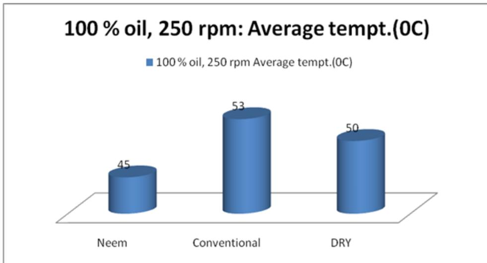
Figure 3. Average Temperatures in (°C) of samples machined with 100% straight oils and dry sample at 250rpm, 1mm depth of cut
