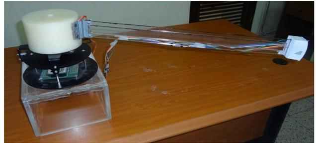
Figure 3. Single link flexible manipulator
