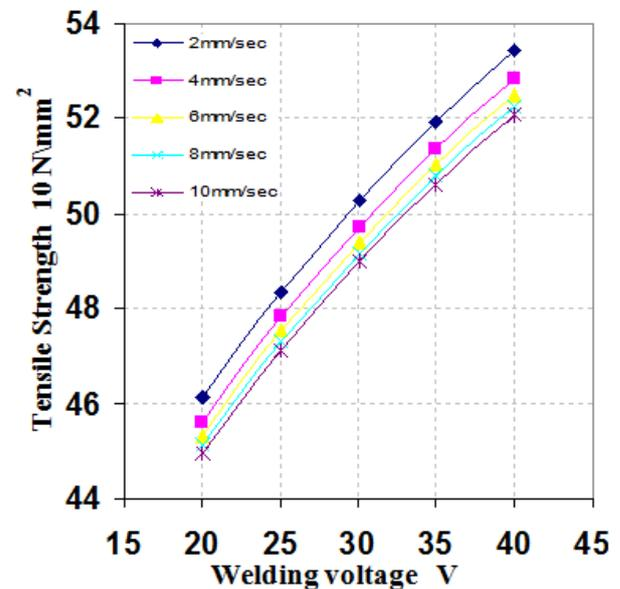
Figure 12-4. Effect of welding voltage and welding speed on the tensile strength at WFR=9m/min, and T=400 °C
