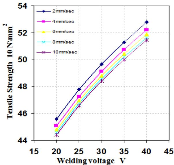
Figure 12-5. Effect of welding voltage and welding speed on the tensile strength at WFR=11m/min, and T=500 °C
