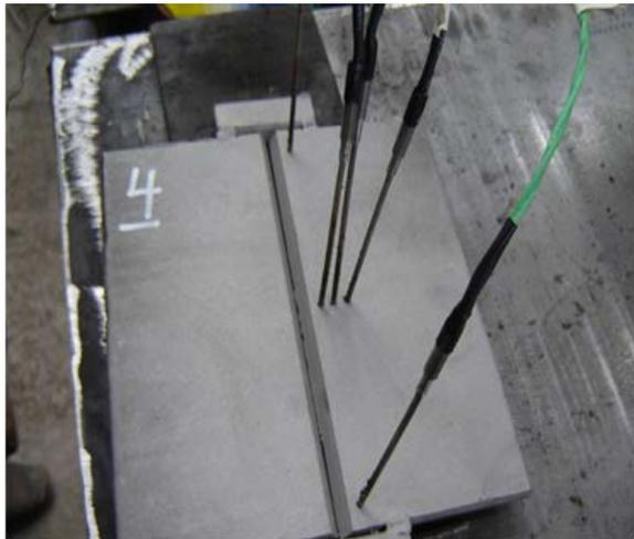
Figure 4. Thermocouples locations in the weld test plate practically in the two-dimension
