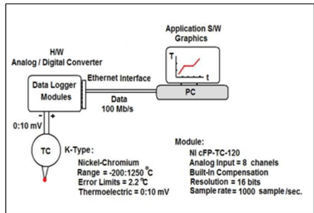
Figure 6. Ethernet interface for compact field point
