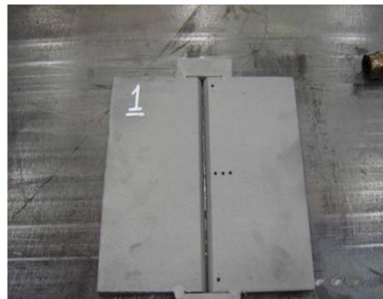
Figure 2. Prequalified CJP of S-V-groove butt weld for the present work
