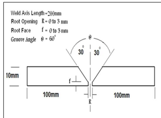
Figure 1. Welded joint details of S-V-groove butt weld (1G position) according to AWS code
