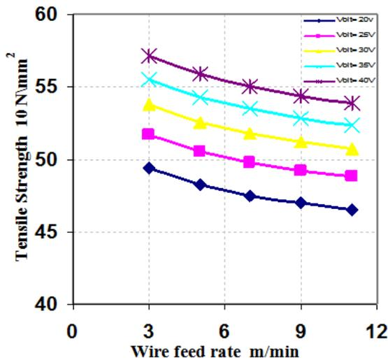
Figure 11-1. Effect of wire feed rate and welding voltage on the tensile strength at S=2mm/sec, and T=100 °C
