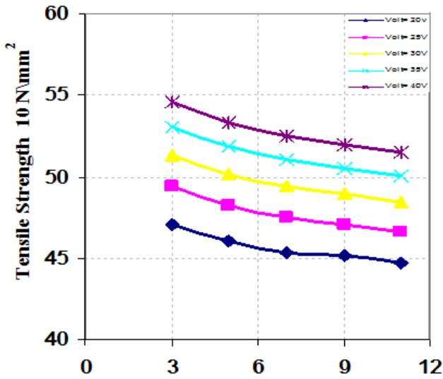
Figure 11-5. Effect of wire feed rate and welding voltage on the tensile strength at S=10mm/sec, and T=500 °C
