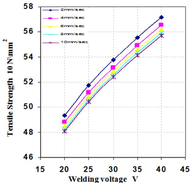
Figure 12-1. Effect of welding voltage and welding speed on the tensile strength at WFR=3m, a/min, and T=100 °C
