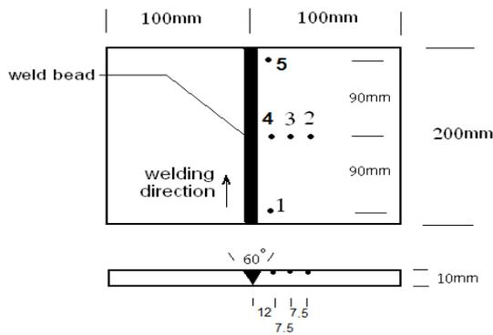
Figure 3. Thermocouples locations and distances between them for the present experimental work in the two-dimension
