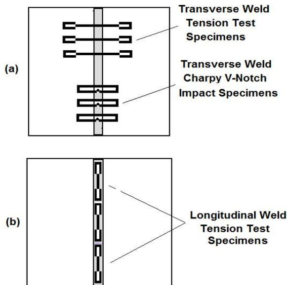
Figure 9. Locations of the tension and impact test specimen according to ASTM code
