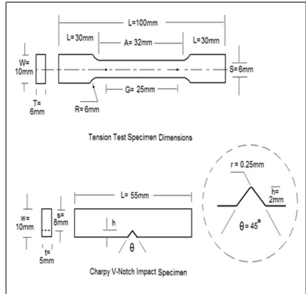
Figure 10. Dimensions of tension and impact test specimen according to ASTM code
