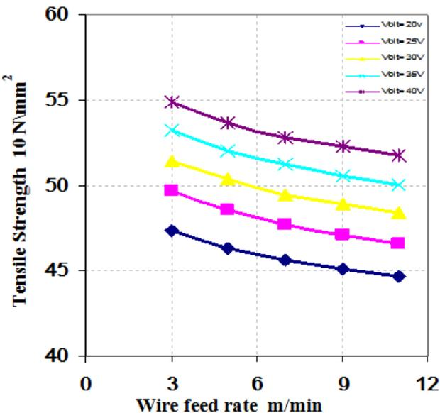
Figure 11-4. Effect of wire feed rate and welding voltage on the tensile strength at S=8mm/sec, and T=400 °C
