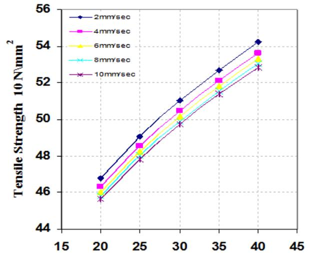
Figure 12-3. Effect of welding voltage and welding speed on the tensile strength at WFR=7m/min, and T=300 °C
