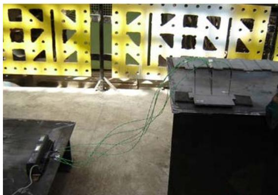
Figure 5. Thermocouples connections with the A/D C modules in the present experimental work
