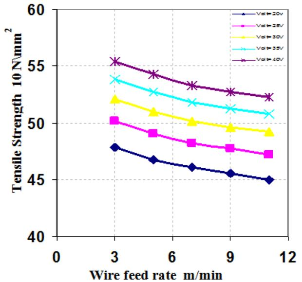
Figure 11-3. Effect of wire feed rate and welding voltage on the tensile strength at S=6mm/sec, and T=300 °C
