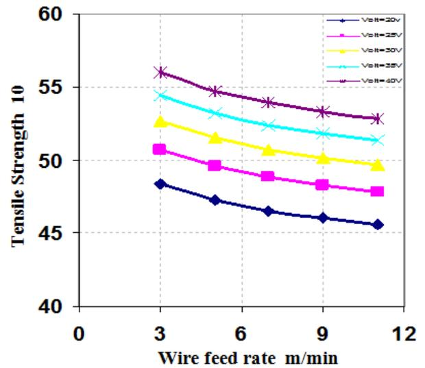
Figure 11-2. Effect of wire feed rate and welding voltage on the tensile strength at S=4mm/sec, and T=200 °C
