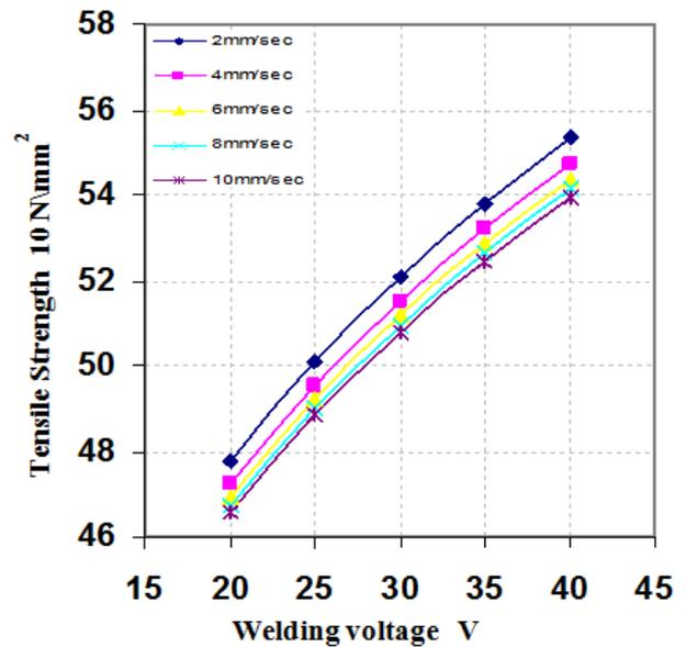
Figure 12-2. Effect of welding voltage and welding speed on the tensile strength at WFR=5m/min, and T=200 °C
