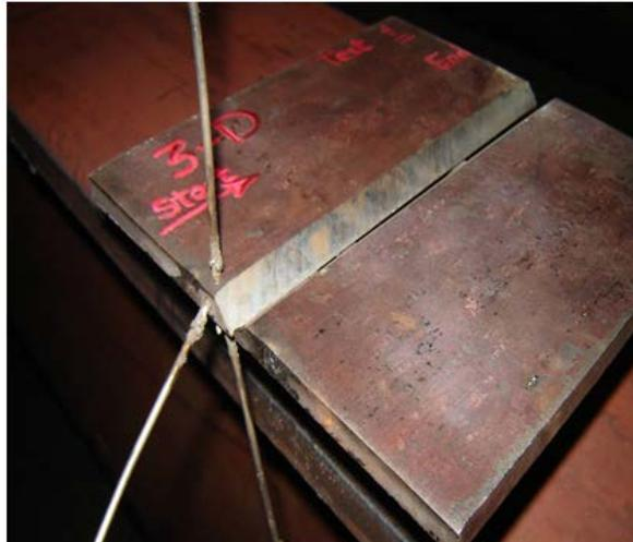
Figure 8. Thermocouples locations in the weld test plate practically in the three-dimension
