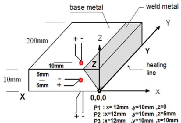
Figure 7. Thermocouples locations and distances between them for the present experimental work in the three-dimension at three points P1,P2, and P3
