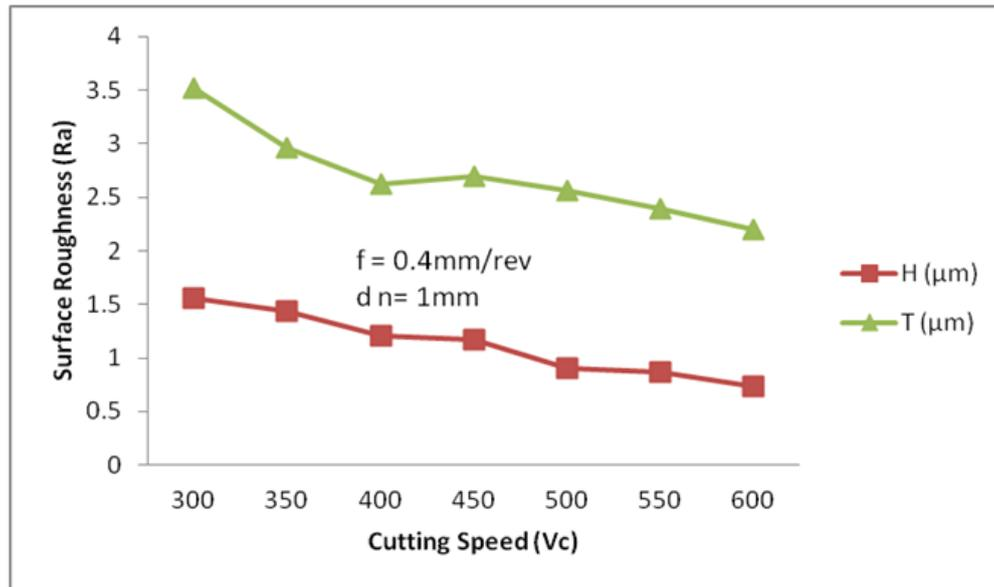
Figure 3. Surface roughness against cutting speed at 0.4mm/rev feed rate
