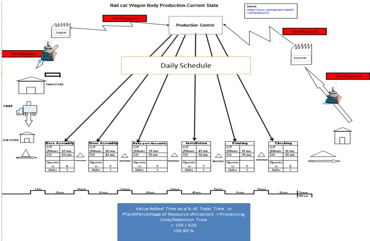
Figure 16. Current Value Stream Mapping for Wagon
