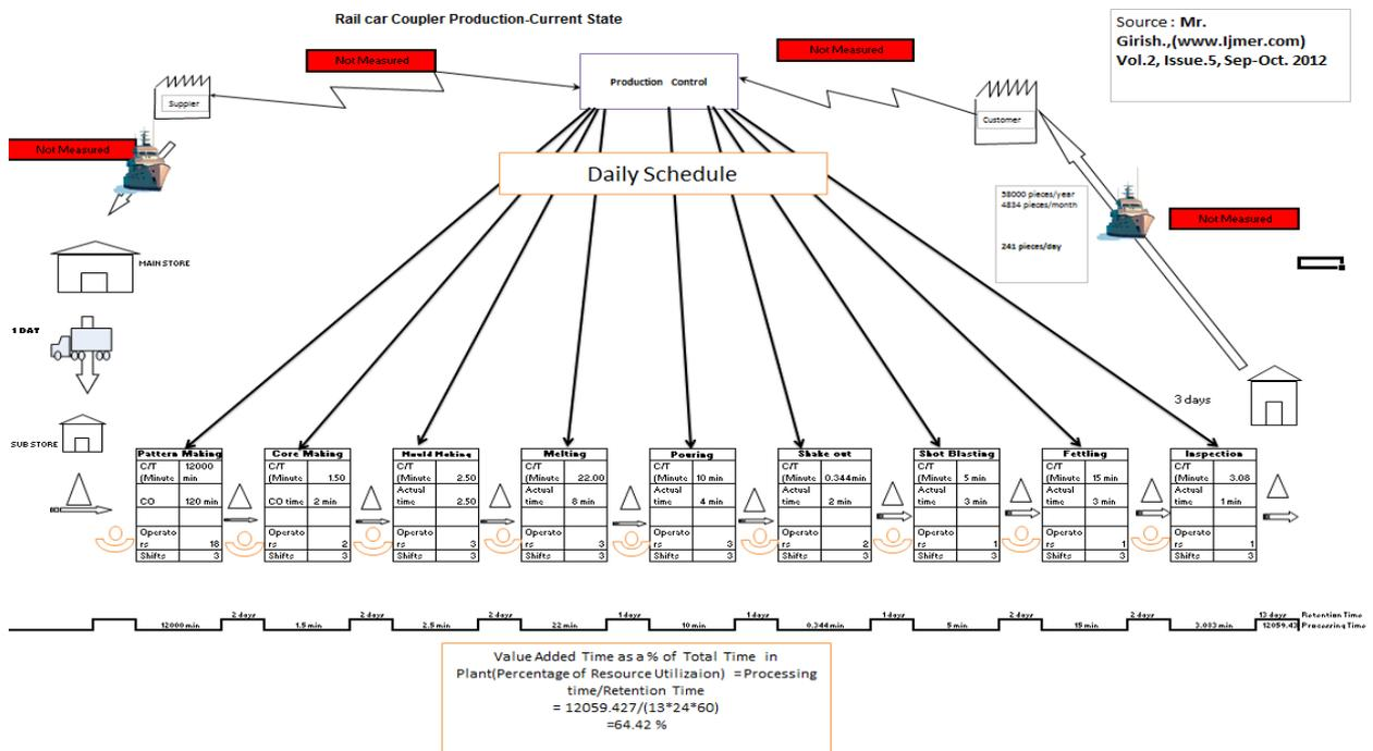
Figure 14. Current State of coupler's VSM
