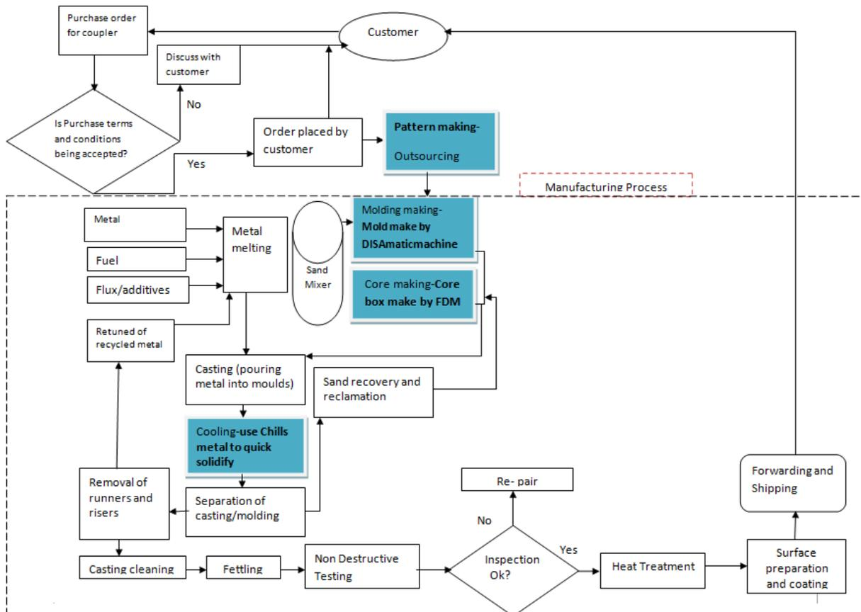
Figure 10. Proposed coupler manufacturing process
