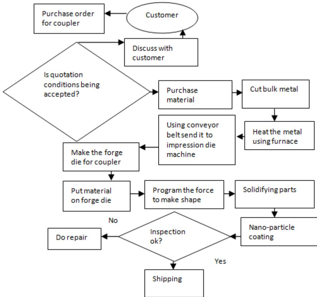
Figure 9. Current coupler manufacturing process flow
