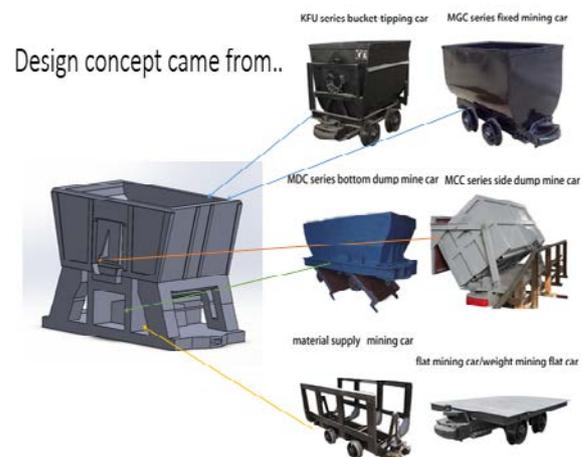
Figure 2. Design concept of multiple way unloading wagon body
