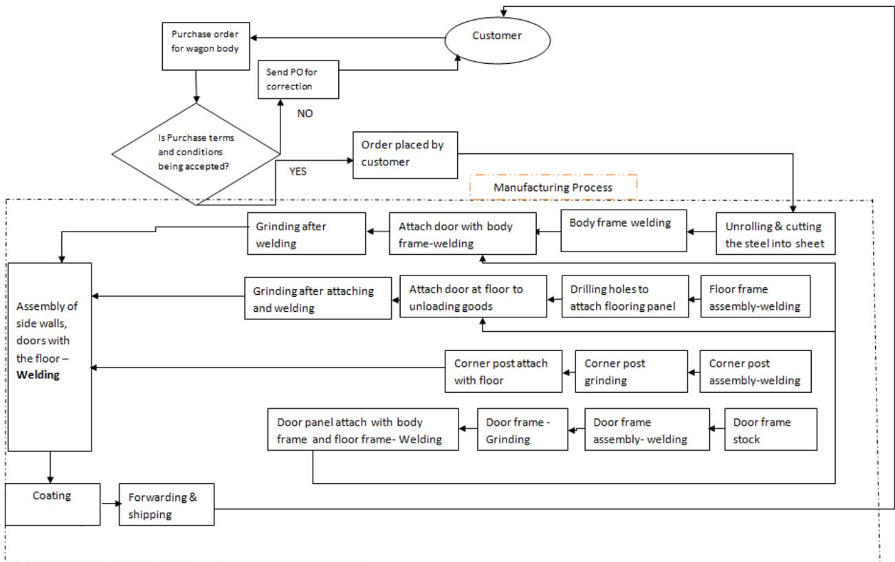
Figure 12. Proposed wagon body manufacturing process flow
