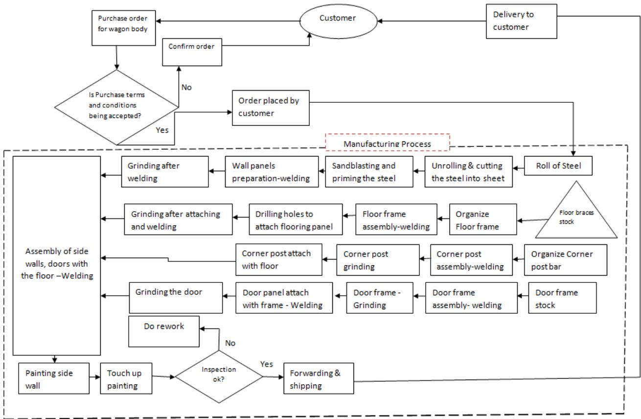
Figure 11. Current wagon body manufacturing process flow
