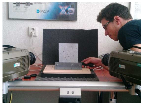
Figure 10. Excitation of the specimen using impact hammer
