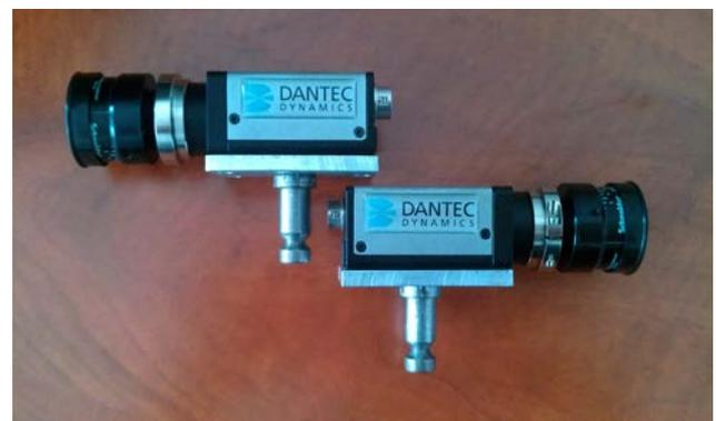
Figure 1. Low-speed CCD cameras of correlation system Q-400 Dantec Dynamics
