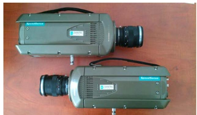
Figure 2. High-speed CMOS cameras of correlation system Q-450 Dantec Dynamics
