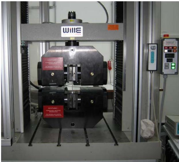
Figure 2. Tensile test machine
