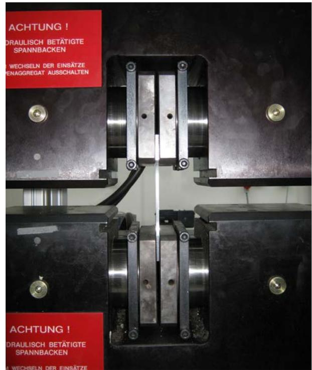
Figure 3. Detail of specimen fixation
