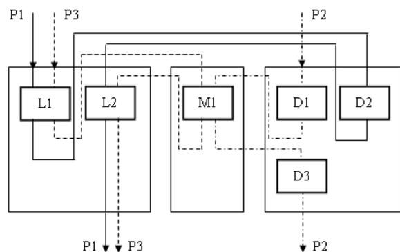
Figure 2. Material flow of the parts P1-P3 in the technological arrangement of the manufacture
