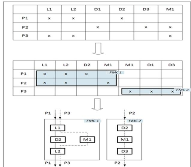
Figure 11. Matrix of troubleshooting machine M1 allocation to each cell
