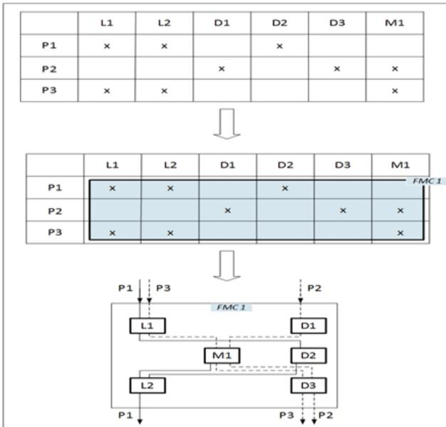
Figure 4. One manufacturing cells for all parts
