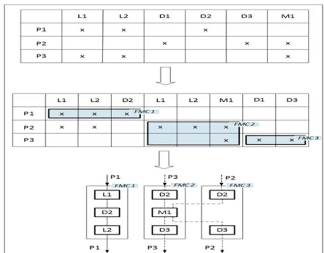
Figure 12. Matrix exploiting the duplicity of machines L1 and L2
