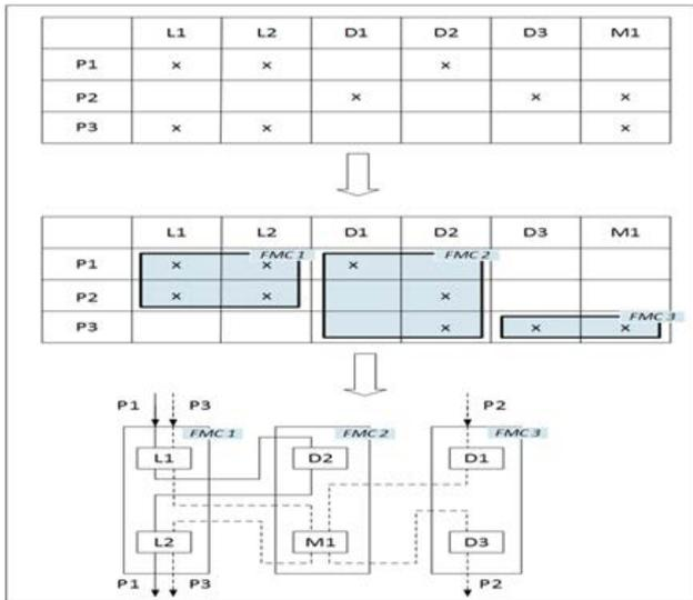
Figure 13. Manufacturing cells with 2 machines
