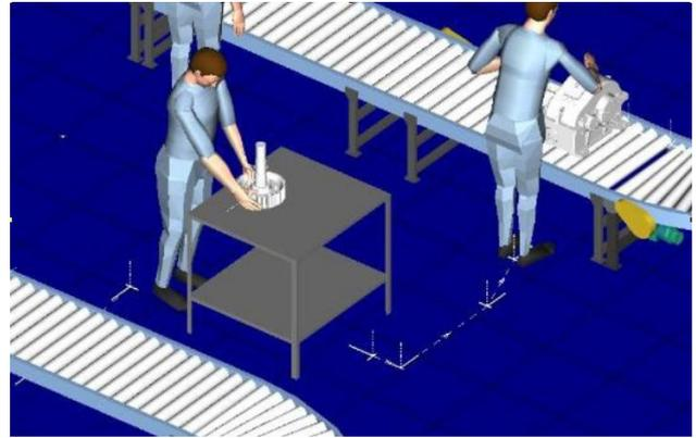
**Figure 5.** Simulation of humans from point of view ergonomics using Tecnomatix Process Simulate
