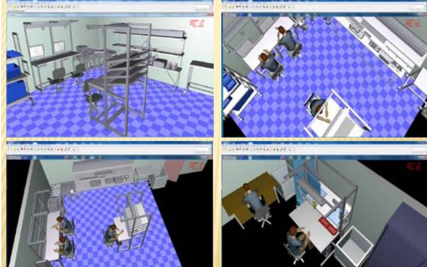
**Figure 3.** Designing of laboratory layout in modular engineering software tool Tecnomatix Process Designer
