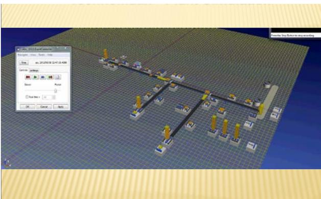
**Figure 4.** Simulation of assembly process in modular engineering software tool Tecnomatix Process Simulate
