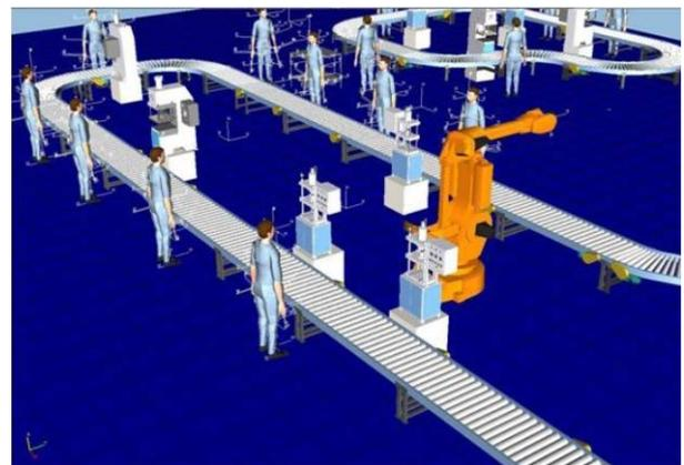
**Figure 2.** Designing of manufacturing layout in modular engineering software tool Tecnomatix Process Designer
