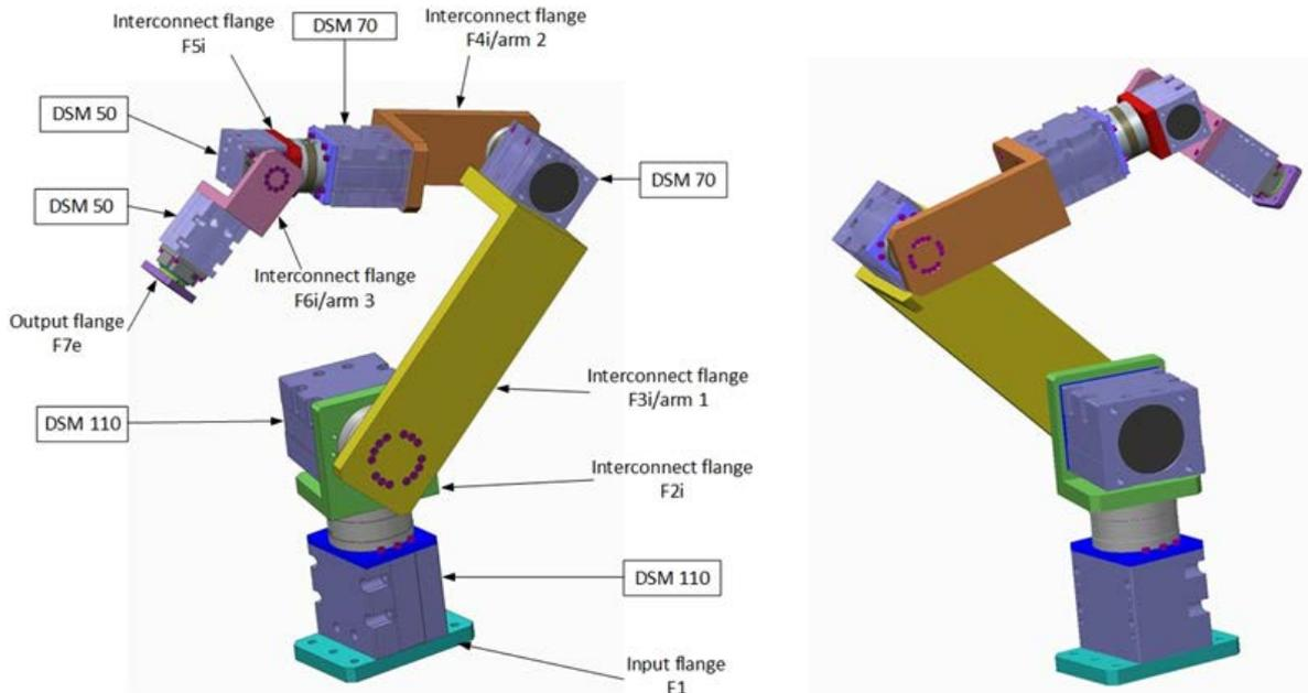
Figure 4. Kinematic structure of modular robotic arm from DSM modules
