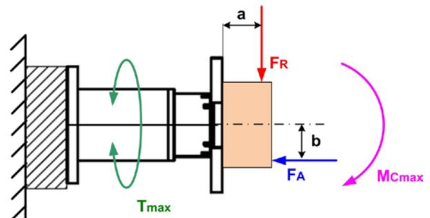
Figure 3. Illustration of the load forces and torques
