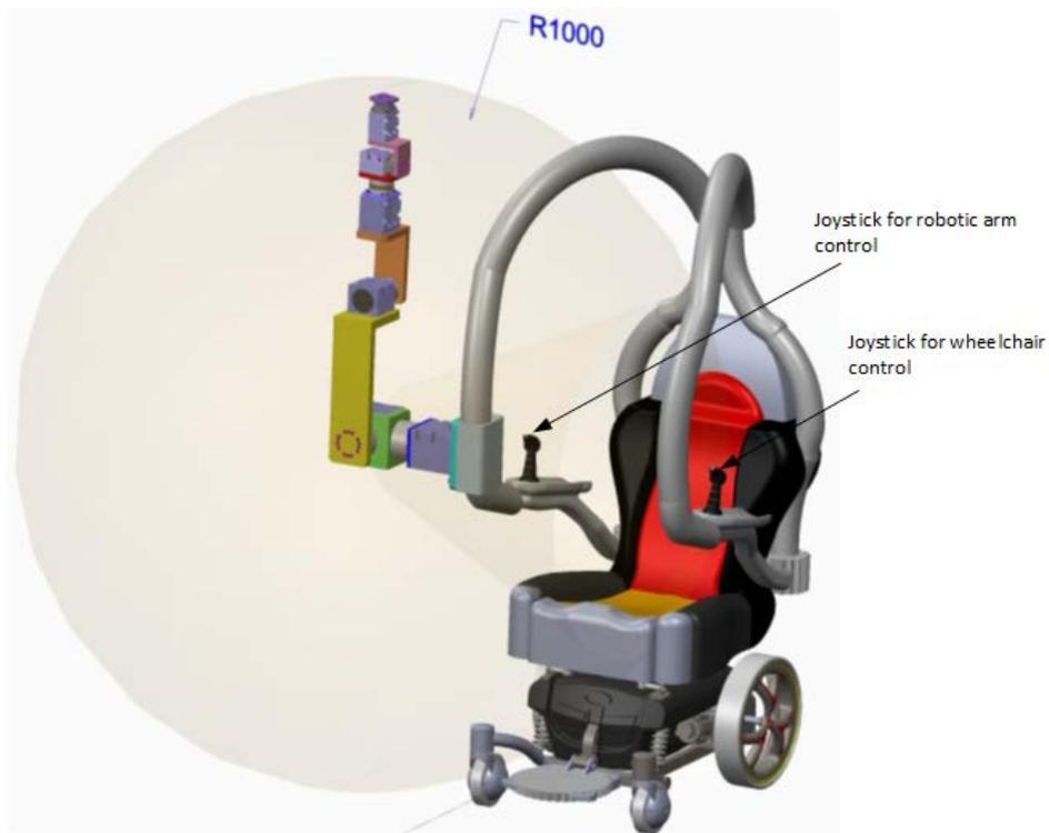
Figure 5. Wheelchair with modular robotic arm
