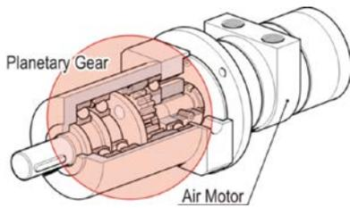
Figure 14. Air motor with integrated gearbox [6] edited by the author
