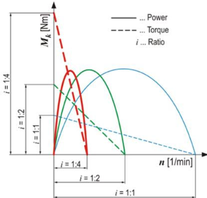
Figure 15. The effect of adding the gearbox to air motor on its characteristics [1] edited by the author
