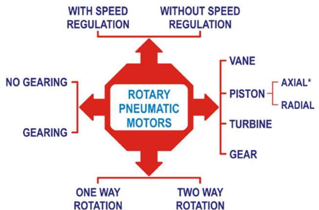
Figure 1. The possibility splitting of rotary air motors
