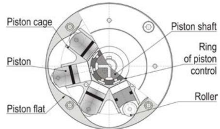
Figure 5. Multi-stroke radial piston air motor [2] edited by the author
