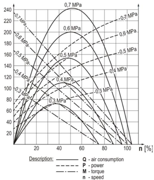
Figure 10. Effect of the operating pressure on the drive parameters [3] edited by the author
