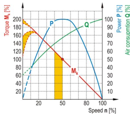
Figure 12. Determination of working point of air motor [6] edited by the author
