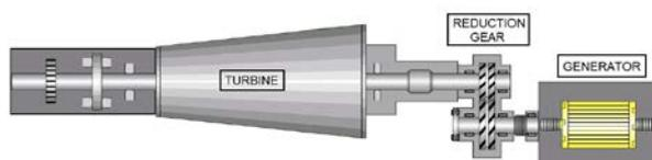
Figure 2. Schema of steam turbogenerator
