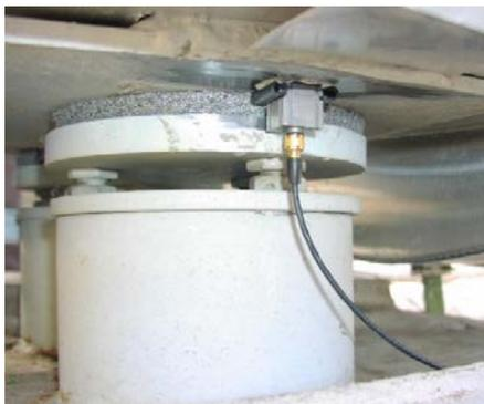
Figure 7. Detail view of applied vibro-isolation mat and triaxial acceleration sensor
