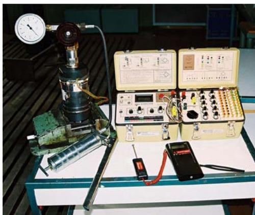
**Figure 10.** The complete set of pressurizing and measuring system for determining processing and functional characteristics of the filling substance
