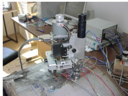
Figure 2. Determination of residual stresses in proximity of weld joint on a sample of pipeline of compressor station
