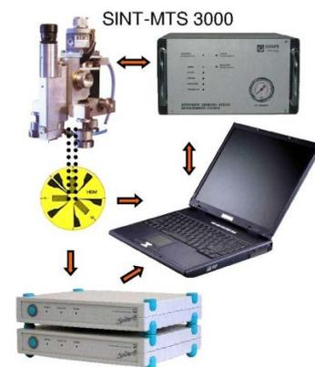
Figure 4. Experimental measuring chain for determining residual stresses by the drilling method using system SINT-MTS 3000
