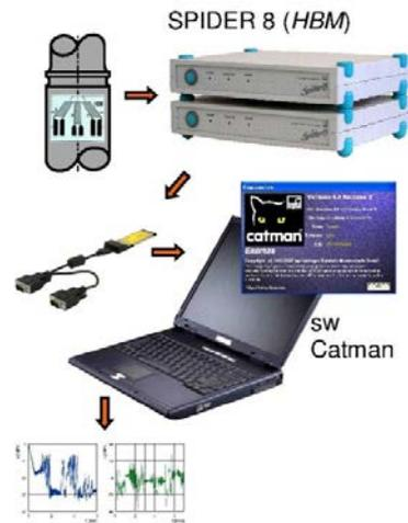
Figure 9. Experimental measuring chain for determining relative deformations using dynamic tensiometric system SPIDER 8
