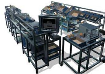
**Figure 3.** Example of modules composed to adaptable manual production system [6]
